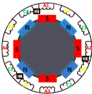
Figure 6. Internal Structure of a BLDC motor [33]
