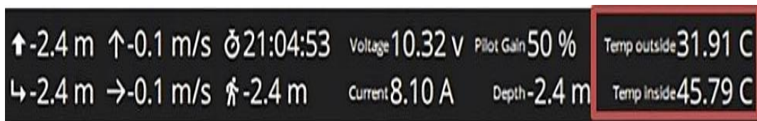
Figure 19. Displays the internal and external temperatures of the Implemented ROV via the QGroundControl software at the bottom of the GUI
