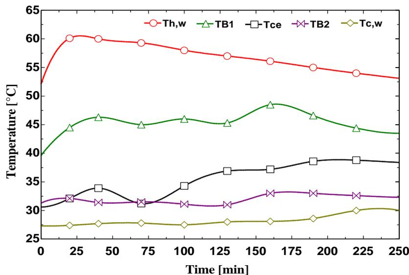
Figure 6. Temperatures of different layers for block filled with cement case.
