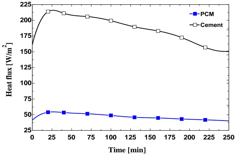
Figure 9. Variation of heat flux with time for PCM and cement.
