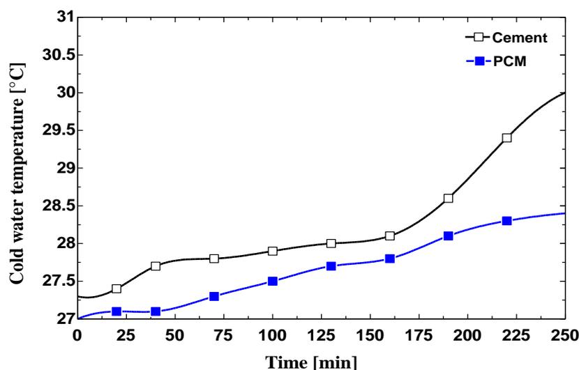
Figure 8. Temperature variation with time for PCM and cement.
