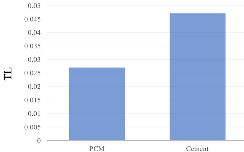
**Figure 11.** Variation in the TLL for the PCM and cement.
