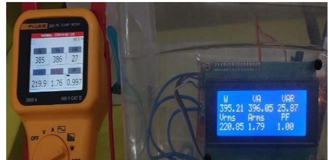
Figure 11. Matching the measurements parameter read by proposed DSMM and Fluke meter for Resistive load.
