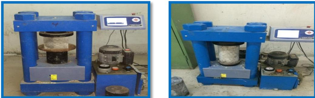
Fig. (5): Concrete Compressive Strength (Cubic and Cylinders)
