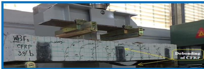
Figure (16): Failure of beam (WBF<sub>1</sub>).
