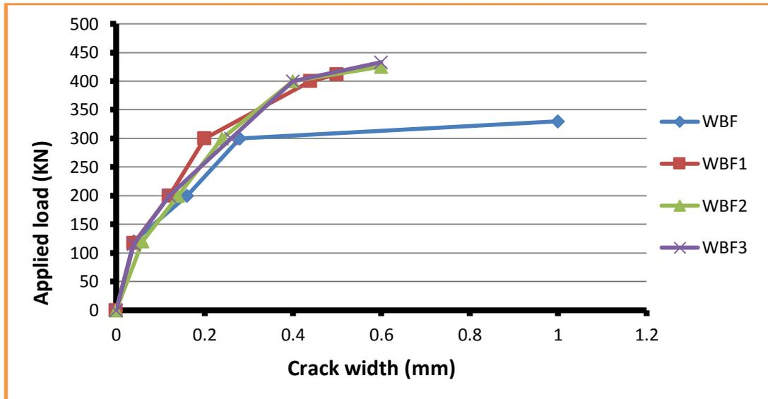
Figure (10): Load\_crack width curve for all tested beams.
