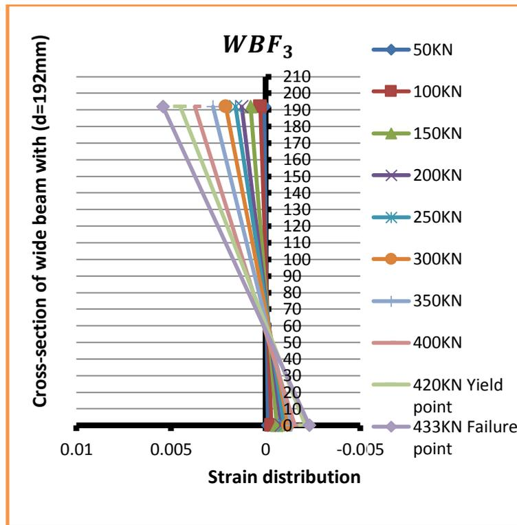
Figure (14): Strain profile for beam ( $WBF_3$ )
