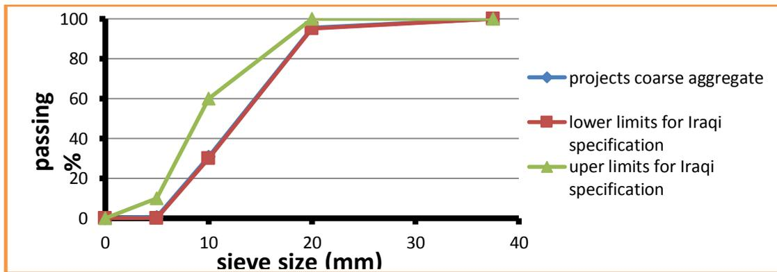
Fig.(3) :Grading of Coarse Aggregate
