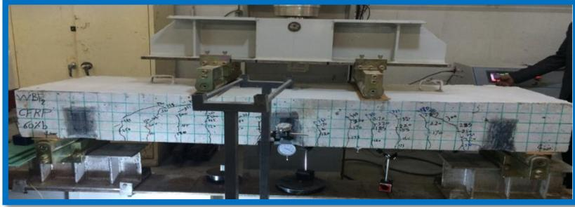
Figure (17): Failure of beam (WBF2).
