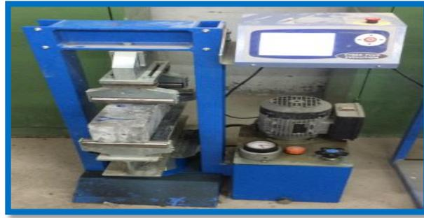
Fig. (7): Modulus of Rupture Test
