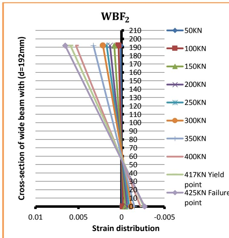
Figure (13): Strain profile for beam (WBF<sub>2</sub>).
