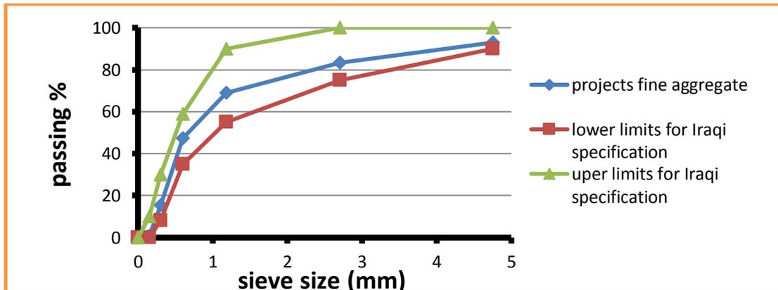
Fig. (2) : Grading of fine aggregate
