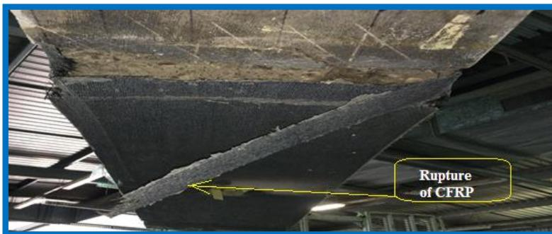
Figure (18): Failure of beam (WBF3).
