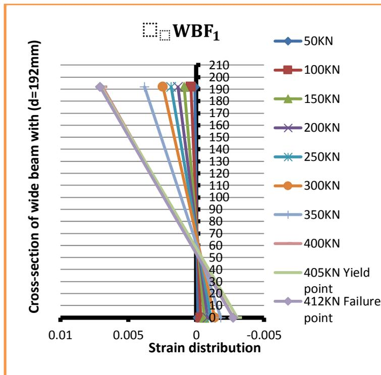
Figure (12): Strain profile for beam (WBF<sub>1</sub>).
