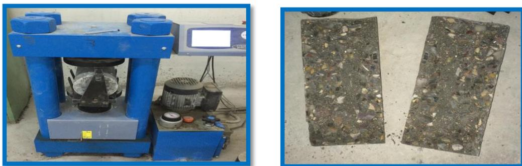
Fig. (6): Splitting Tensile Strength Test
