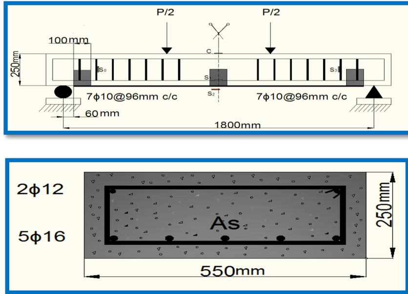
Figure (1): Typical dimensions and details of tested beams
