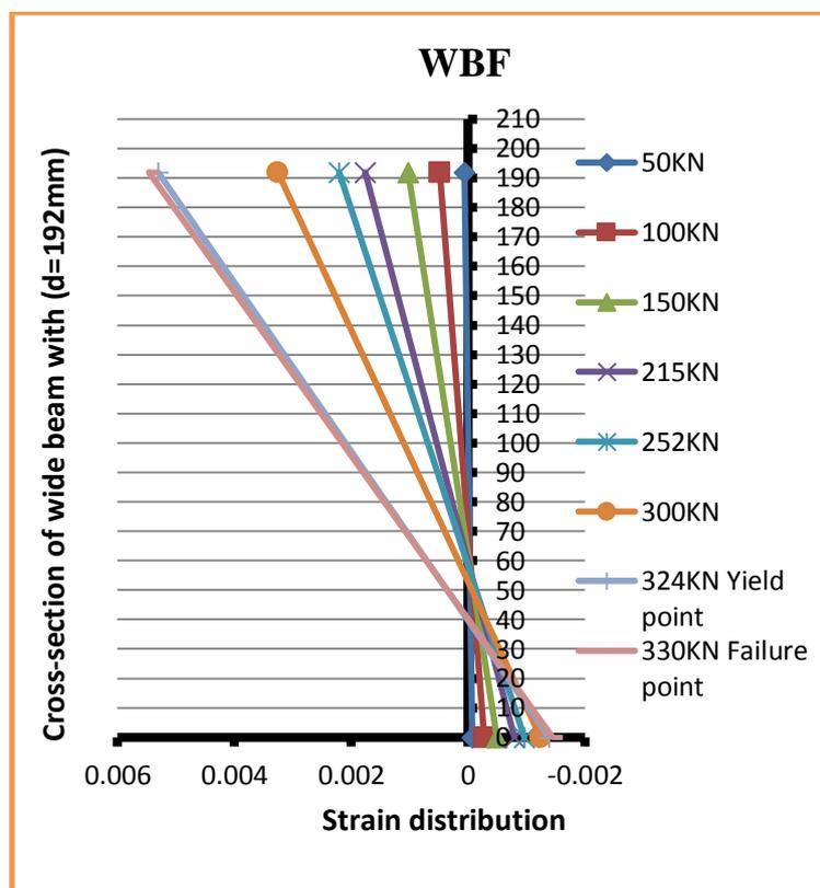
Figure (11): Strain profile for beam (WBF).
