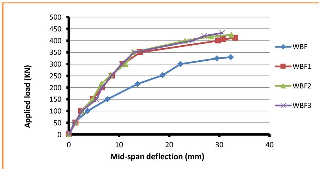
Figure (9): Load\_ deflection curve for all tested beams.
