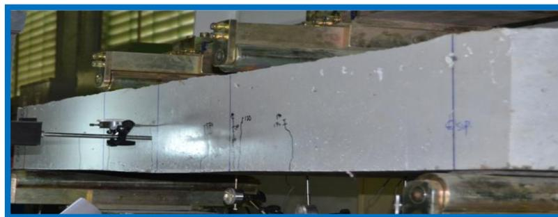
Figure (15): Failure of beam (WBF).
