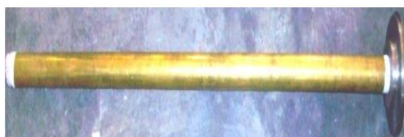
Figure 2. Photograph of inner tube or HTF tube with a circular plate
