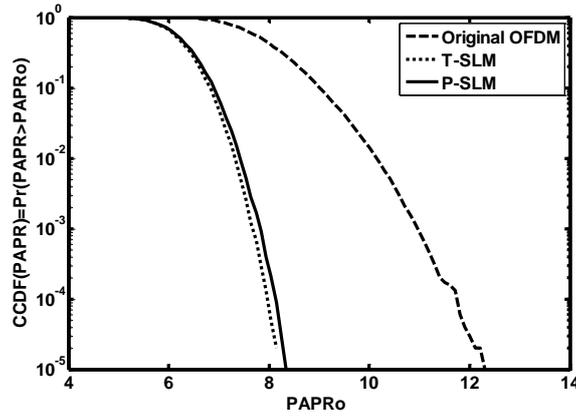
**Fig. 3(a):** PAPR reduction performance of P-SLM and T-SLM for  $U=16$ ,  $L=4$ , and 64-PSK modulated OFDM signal with  $N=256$
