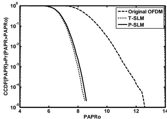
**Fig. 3(b):** PAPR reduction performance of P-SLM and T-SLM for  $U=16$ ,  $L=4$ , and 64-PSK modulated OFDM signal with  $N=512$
