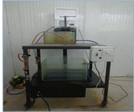
Fig. (2): Experimental set up of ECM .process
