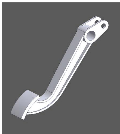
Figure 2. Baseline simplified CAD model of the brake pedal showing key functional features.
