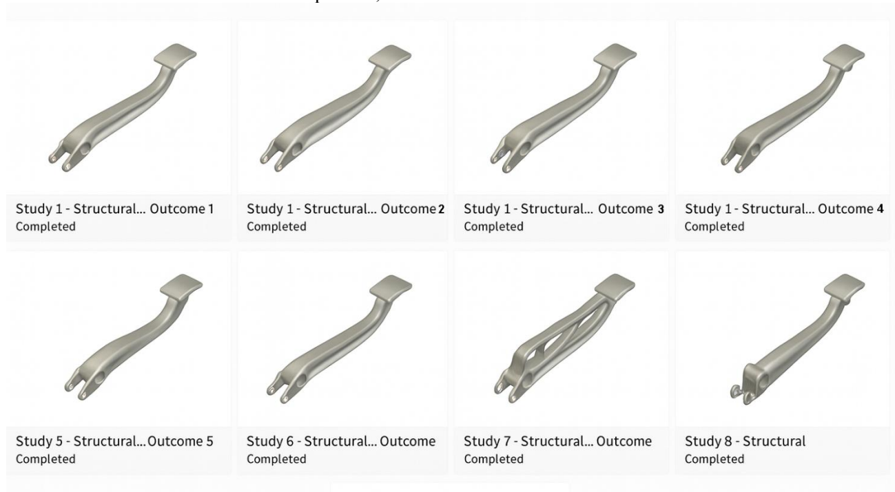
Figure 5. Generative design outcomes for the brake pedal under additive, machining, and die-casting constraints.
