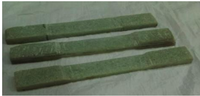
Figure 6. Tensile samples (a) ASTM Figure D3039 standard dimensions [38], (b) Fabricated coupons.
