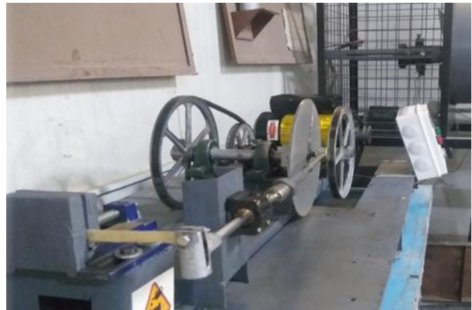
Figure 7. Fatigue specimens, (a) Standard dimensions [23], (b) Fabricated specimens, (c) Reciprocating bending fatigue machine
