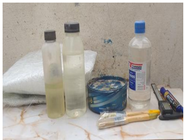
Figure 5. Materials used in lamination of composite plate, 1- short glass Fiber, 2- Hardener, 3- Polyester 4- Insulating wax, 5- Thinner 6- Brushes, vernier and permanent marker
