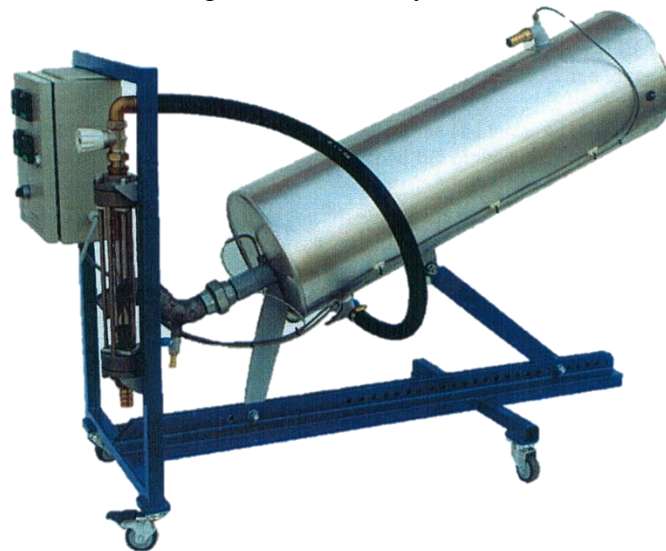
Fig. (3): The exhaust gas calorimeter unit.
