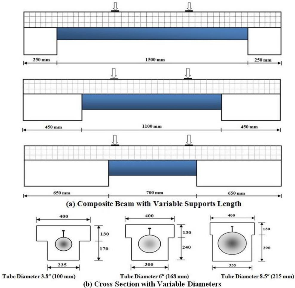
Figure (1) Typical Geometry of Test Specimen
