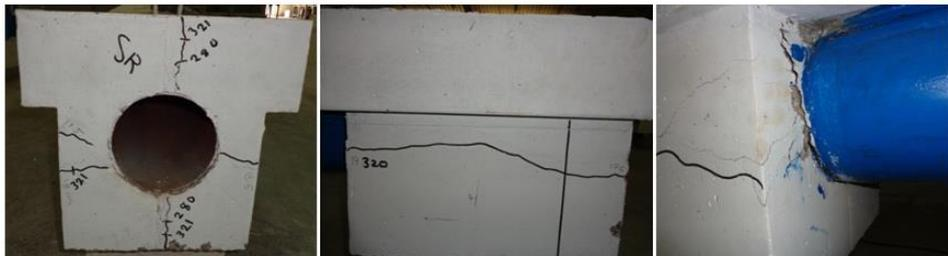
Crack around steel tube      Longitudinal crack at support      Crack from inner to outer
