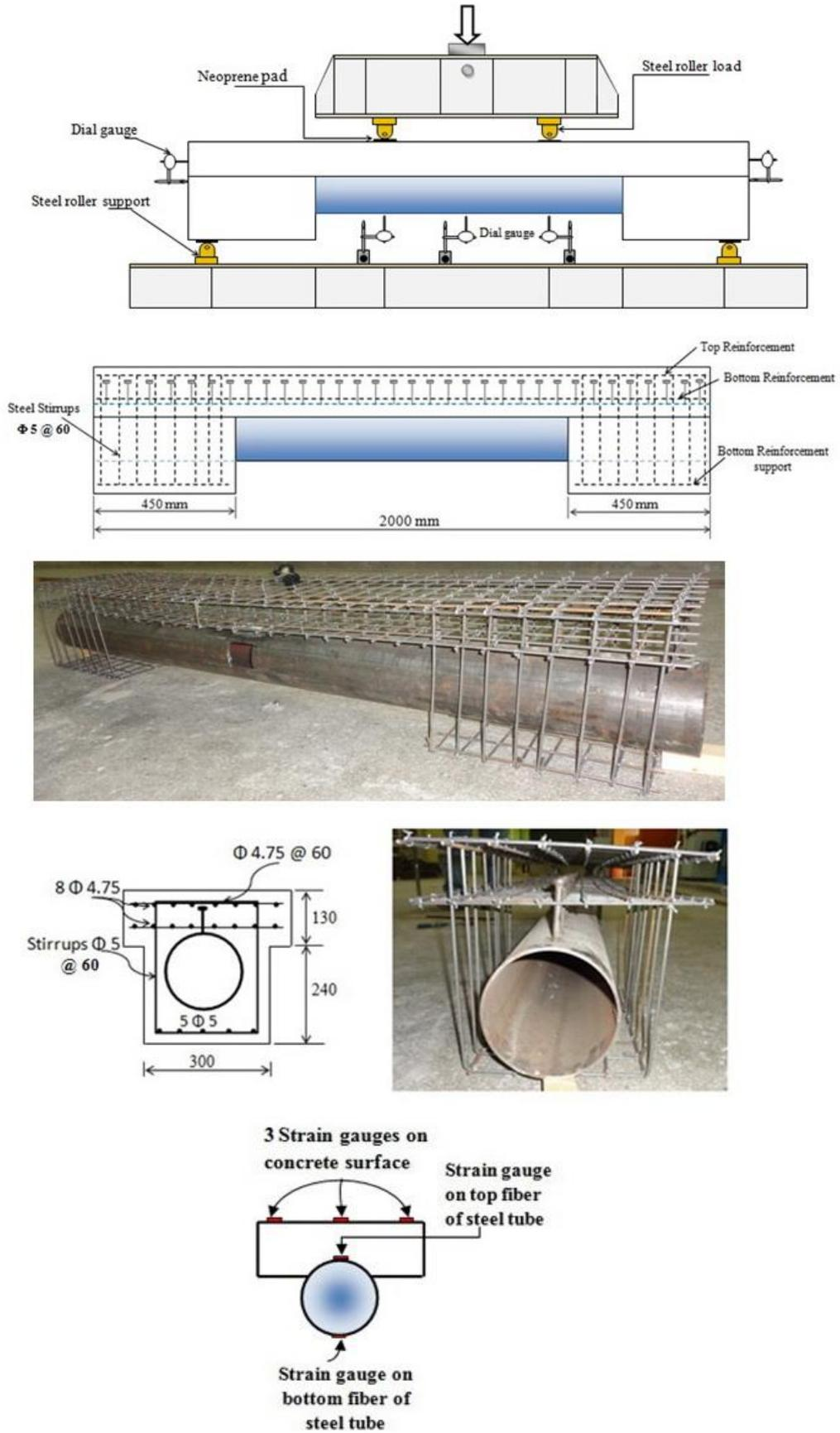
Figure (2) Test Specimen Beam
