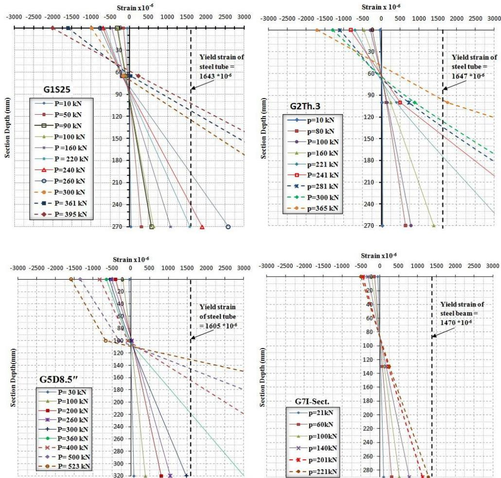
Figure (8) Strain profiles of Specimens
