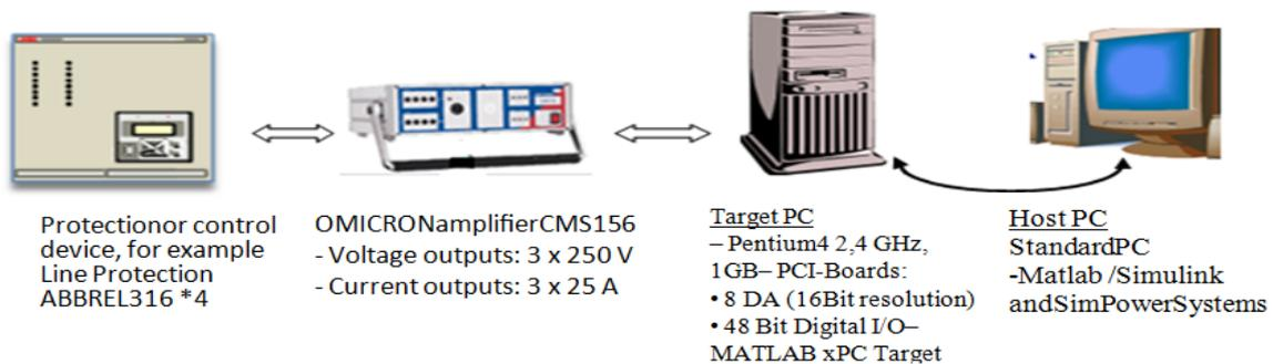
Figure (1): Components in the real-time simulation for a protective device
