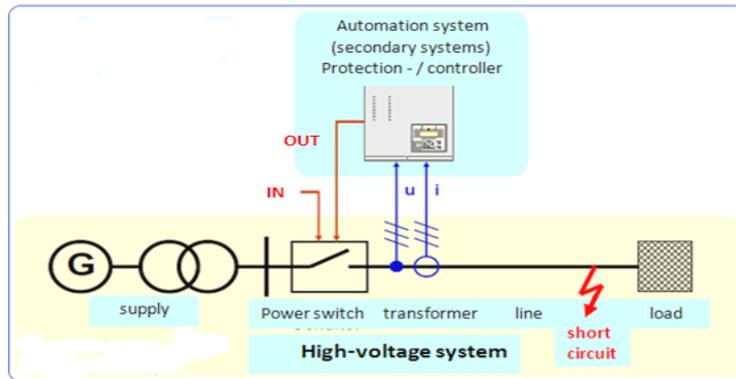
Figure (4) primary and secondary equipment in the line protection
