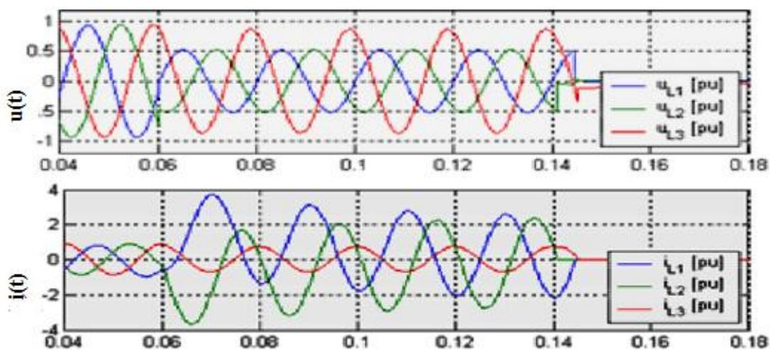
Figure (6) Voltages and currents with a protective response in a 2-pole earth fault
