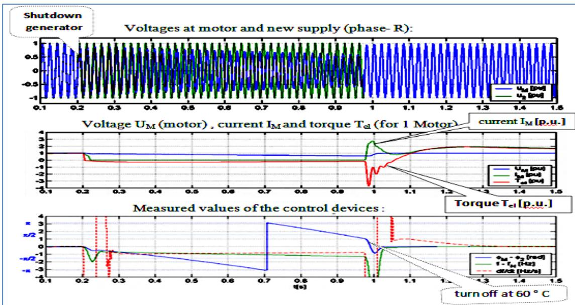
Figure (11): Timing a bus-bar/fast changeover
