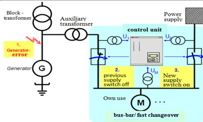
Figure (10) System configuration and control unit for abus-bar fast change-over
