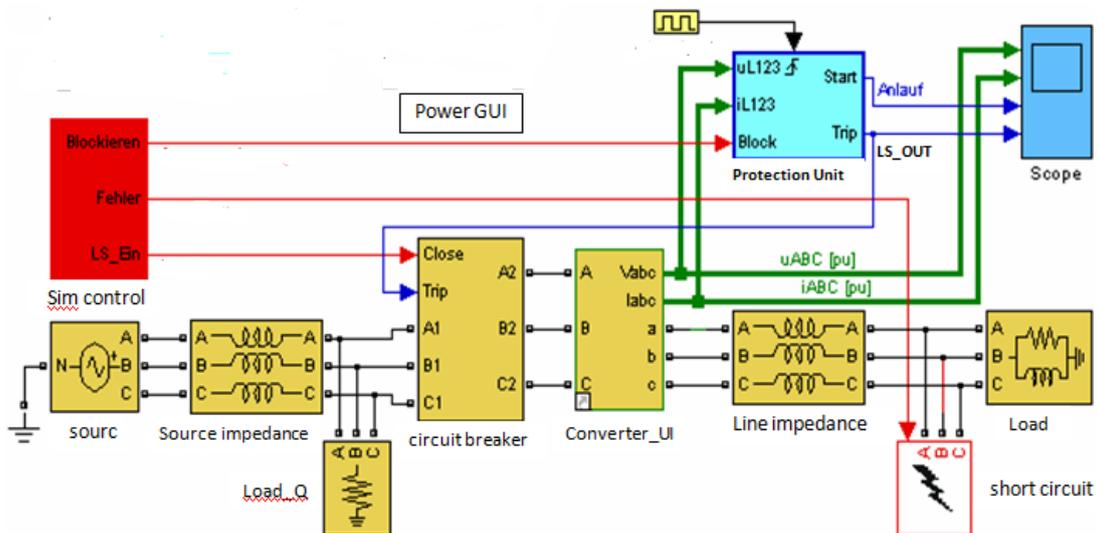
Figure (5) Model of a high-voltage line, with line protection
