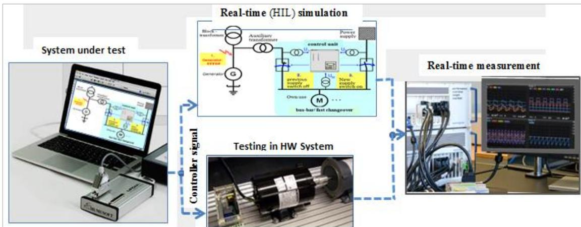
Figure (9) Demonstration of a hardware-in-the-loop (HIL) simulation
