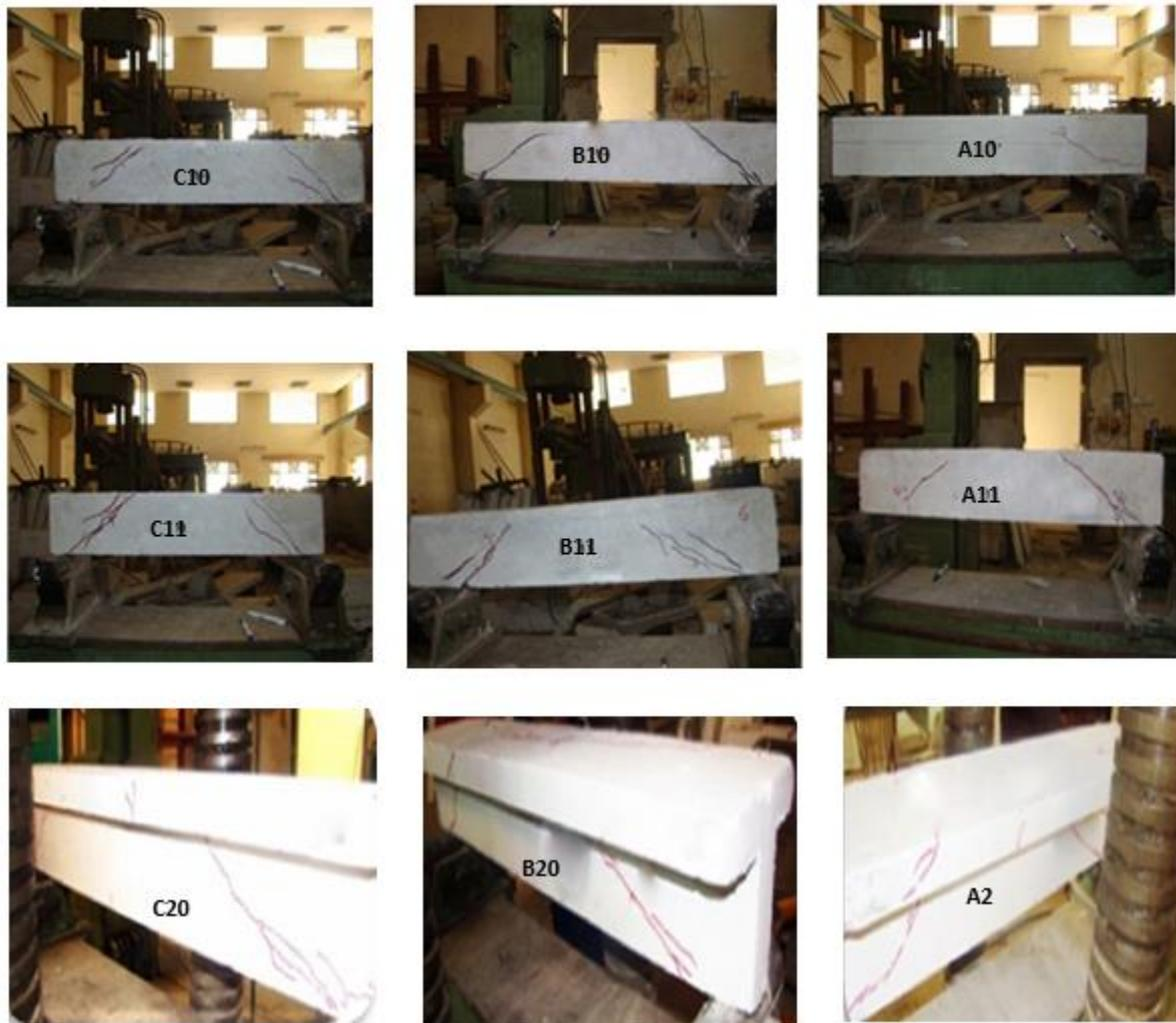
**Fig (17):** Crack pattern of the tested SCC beam specimens
