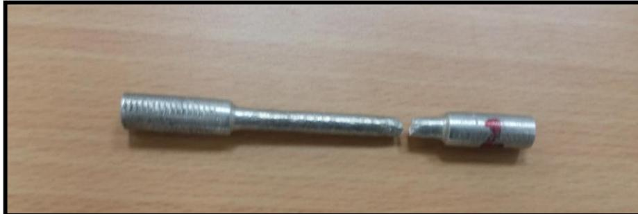
Fig. (3): Tensile specimen after test.
