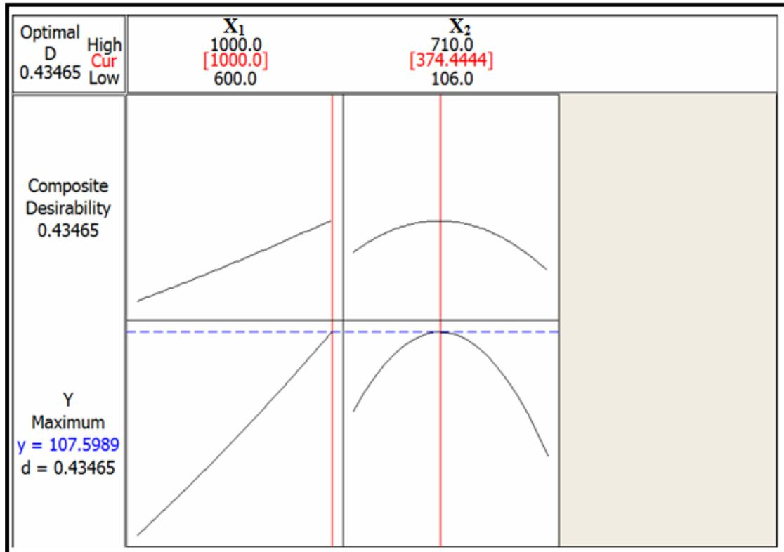
**Fig. (8):** Optimization chart for maximum tensile strength.
