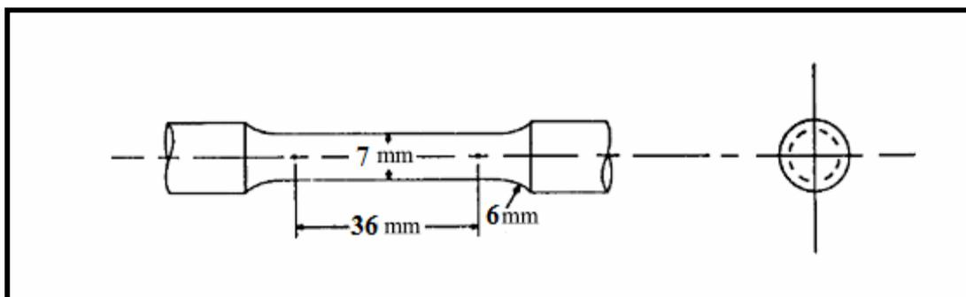
**Fig. (2): ASTM standard tensile specimen.**
