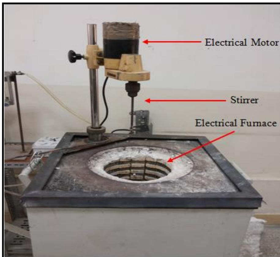
**Fig. (1): Casting stir instrument method**
