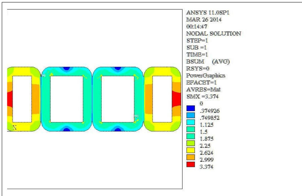
Fig. (21): Contour plot of zero sequence flux density distribution in iron core.
