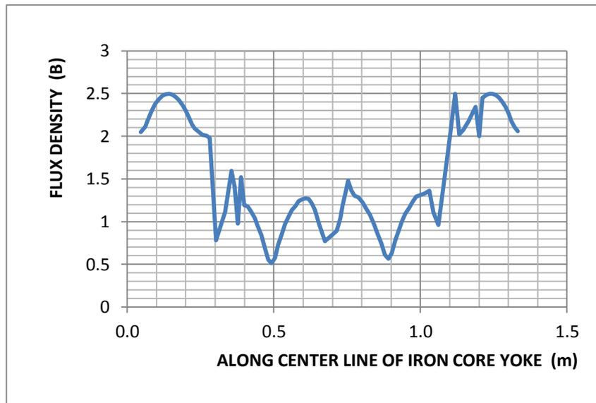
**Fig. (23):** Illustrated the distribution of magnetic flux along the center line of X direction (length of core) at yoke region.
