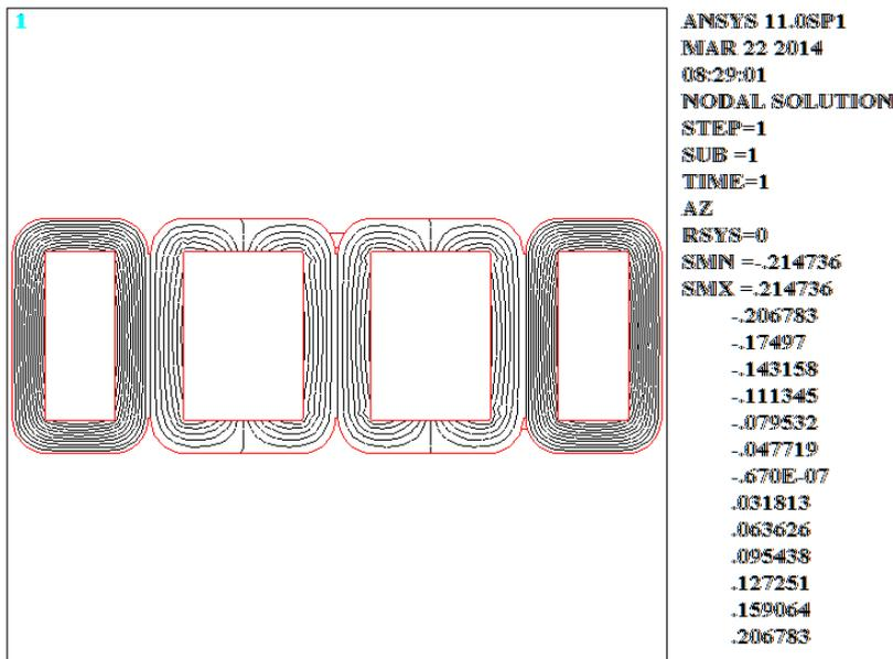
Fig. (19): Zero sequence flux lines distribution in iron core.
