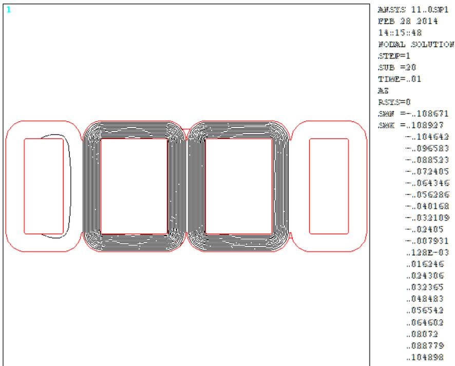
**Fig. (25):** Illustrates the distribution of magnetic flux in core at balanced condition.
