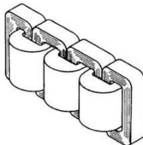
**Fig. (14):** Five-legged wound core-type transformer.
