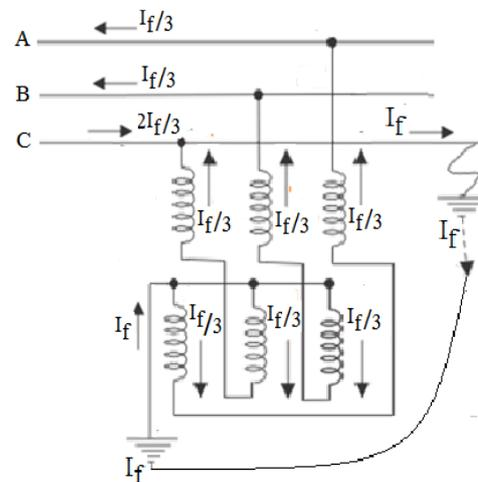
Fig. (5): Earth fault current when single line to ground fault occurs on any phase of the system.
