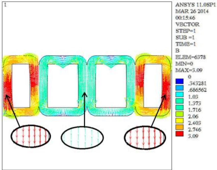
Fig. (20): Zero sequence flux density vectors distribution in iron core.
