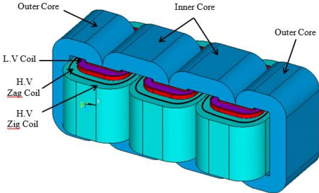
**Fig. (6):** Active part configuration of the zig-zag grounding transformer.
