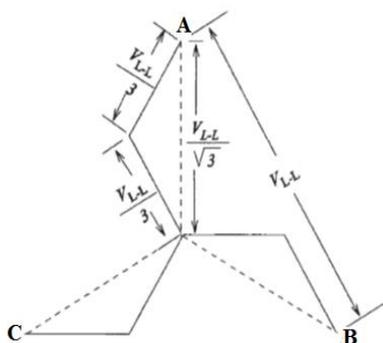
Fig. (4): Vector diagram of a zig-zag transformer connection.
