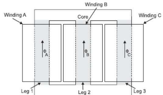
**Fig. (13):** three-legged core-type transformer magnetic paths
