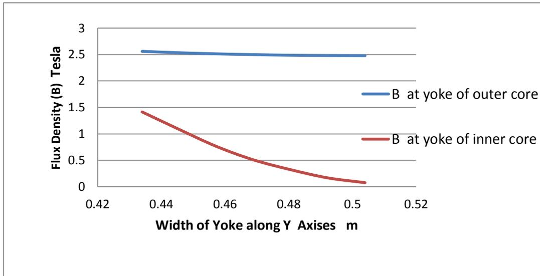
**Fig. (24):** Illustrated the distribution of magnetic flux at width of yoke region (Y axis) region.
