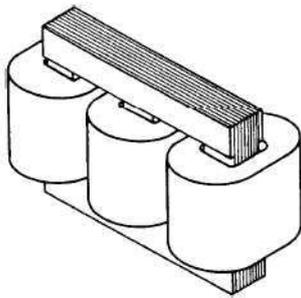
**Fig. (12):** Three-legged core-type transformer.
