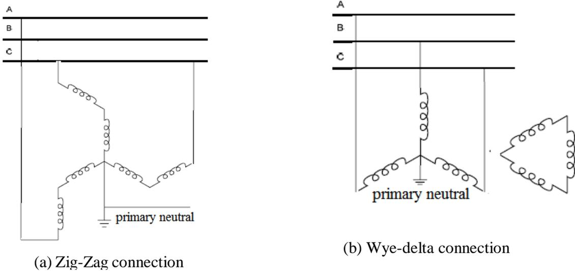
Fig. (1): Grounding transformer connections.
