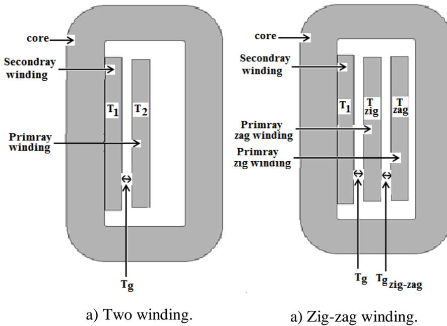
**Fig. (16):** Part sections of two winding and zig- zag transformer.
