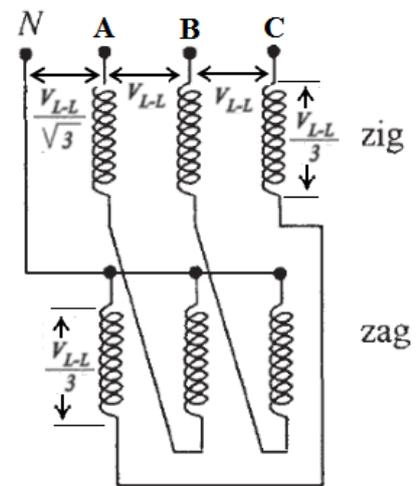
Fig. (3): zig-zag transformer connections.
