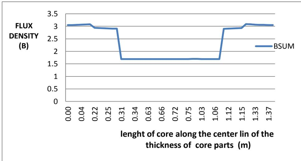
**Fig. (22):** Illustrated the distribution of magnetic flux along the center line of the thickness of wound core parts (outside parts and internal parts).
