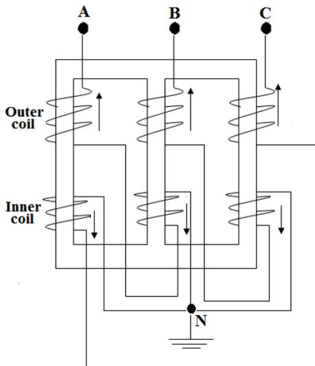
Fig. (2): zig-zag transformer arrangement.
