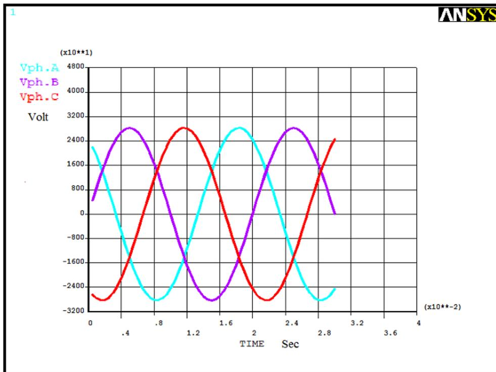
a) Input voltage waveform.
