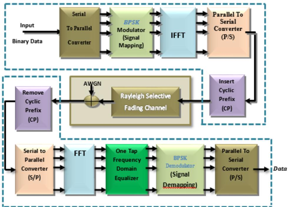
Figure (2): OFDM System Modeling <sup>(6)</sup>
