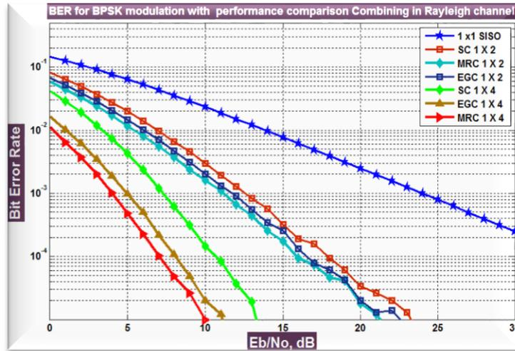
Figure (11): BER performance comparison of SC, EGC and MRC with different number of receive antennas
