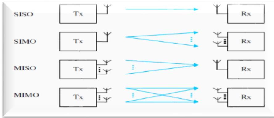
Figure (1) Types of antenna (SISO, SIMO, MISO, and MIMO)
