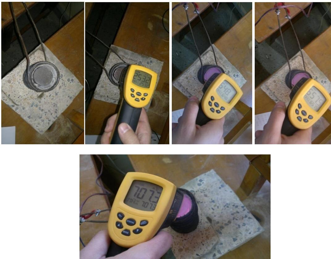
**Figure (14):** It represents the increase in billet temperature, during the heating process.
