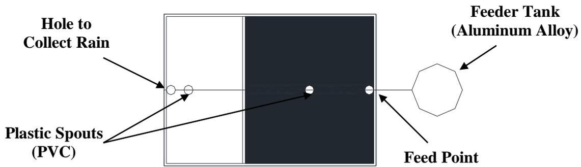
**Fig. (4):** The Designed Still (Top View).
