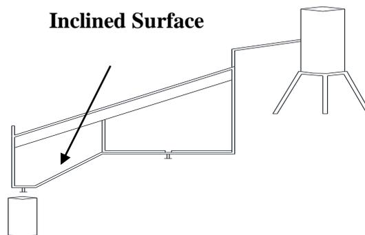
**Fig. (2):** The Designed Still (Front View).
