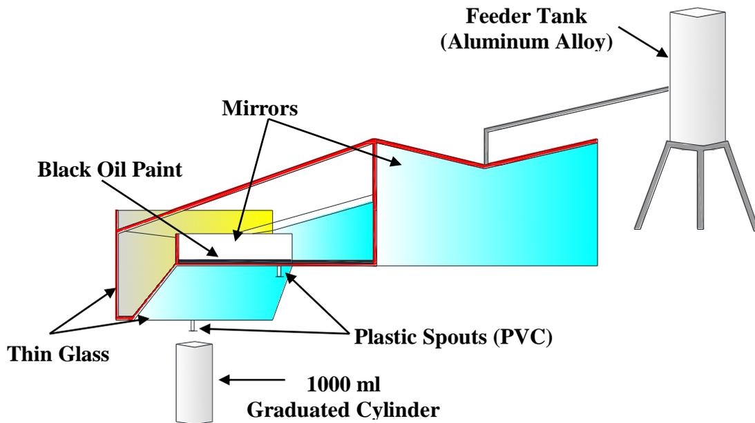
**Fig. (1):** The Designed Still (3D View).
