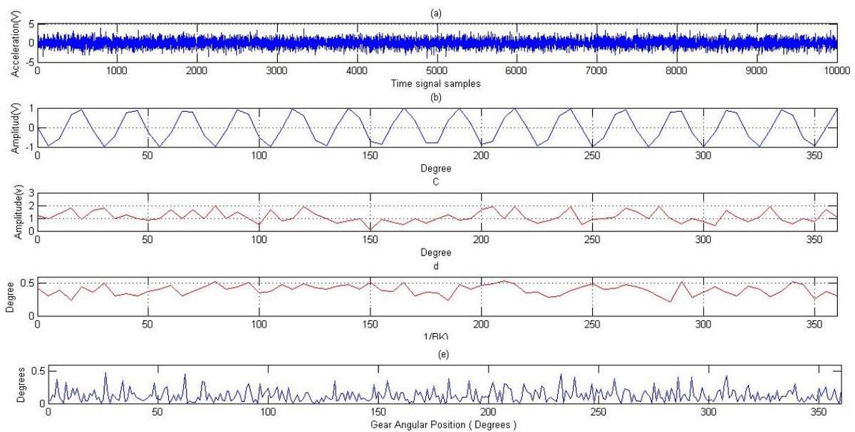
**Figure(3):** Healthy gear processing results : (a) Part of the original vibration signal; (b) Signal average; (c) Wavelet reference function; (d) Beta kurtosis reference function; (e) Phase modulation reference function.
