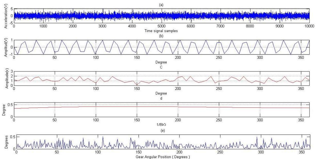
**Figure (4):** Cracked gear processing results: (a) Part of the original vibration signal; (b) Signal average; (c) Wavelet reference function; (d) Beta kurtosis reference function; (e) Phase modulation reference function.
