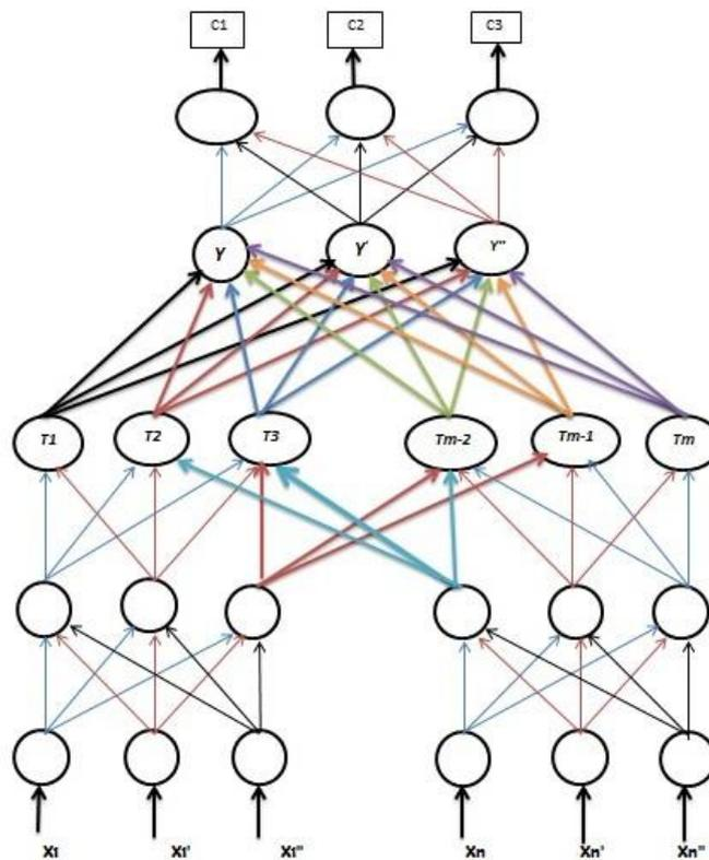
**Figure (2):** The network architecture of the proposed integrated classifier
