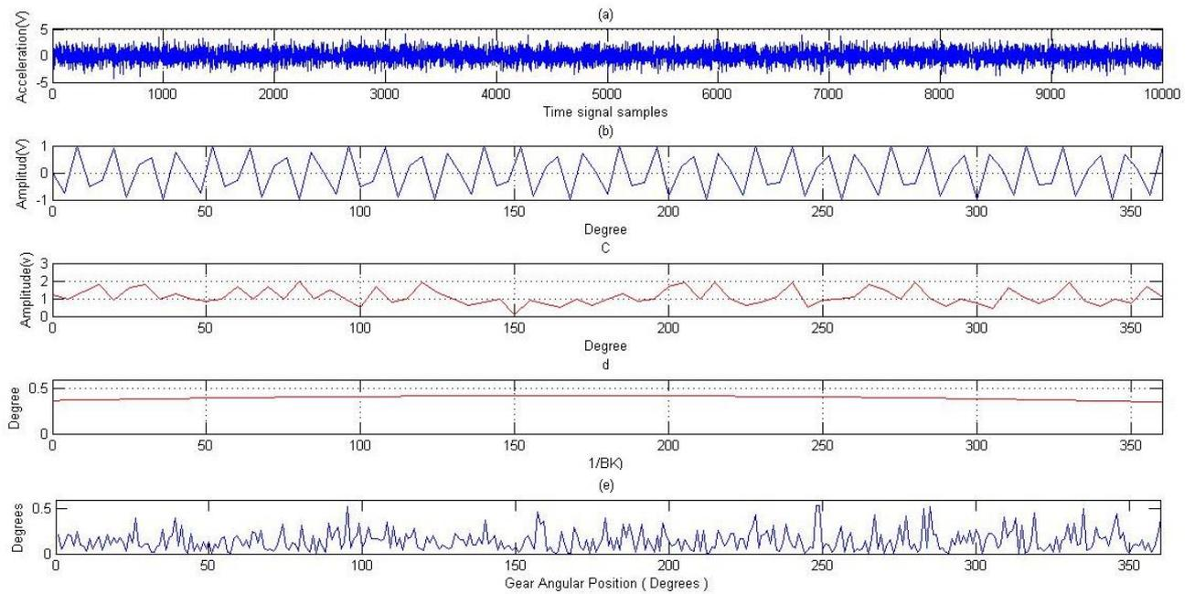
**Figure (5):** Chipped gear processing results: (a) Part of the original vibration signal; (b) Signal average; (c) Wavelet reference function; (d) Beta kurtosis reference function; (e) Phase modulation reference function
