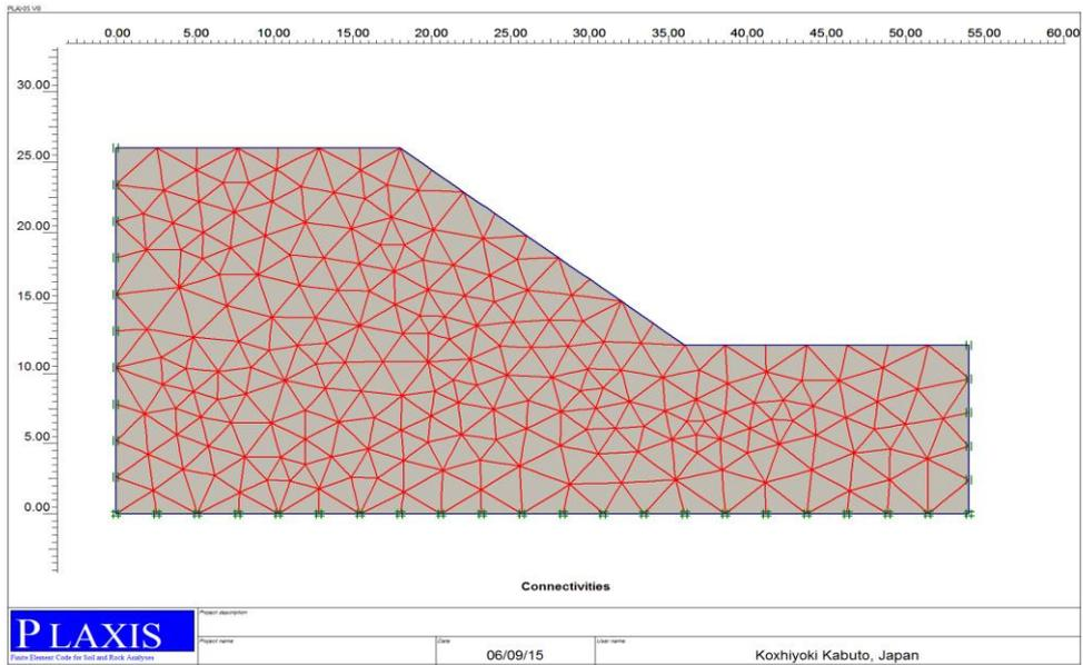
**Figure 2.** Two Dimensional Finite Element mesh
