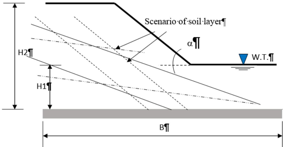
**Figure 1.** Model for the slope
