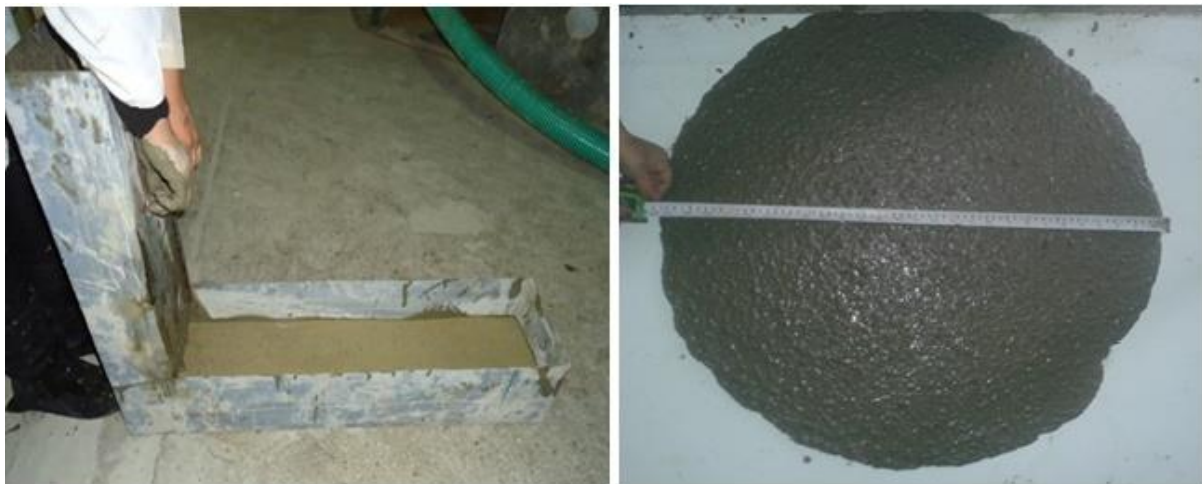
Figure (6) Flowing SCC in L-box test Figure (7) Spreading SCC in slump flow test
