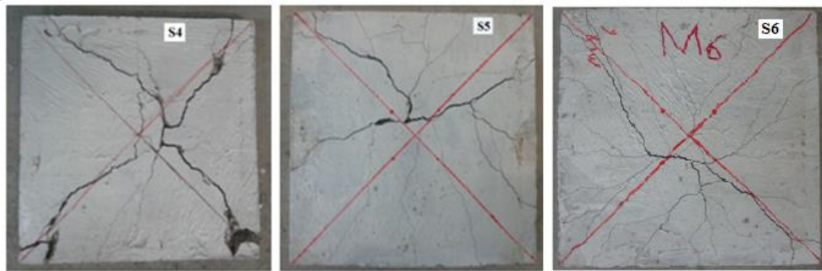
Figure (16) Effect of steel fiber volumetric ratio on crack pattern of high strength SCC slabs
