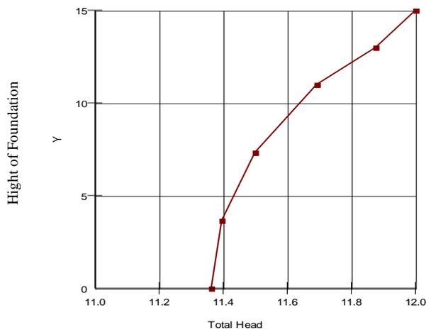
**Fig.(14): Sec. C-C Head of water pressure Vertical section U/S**
