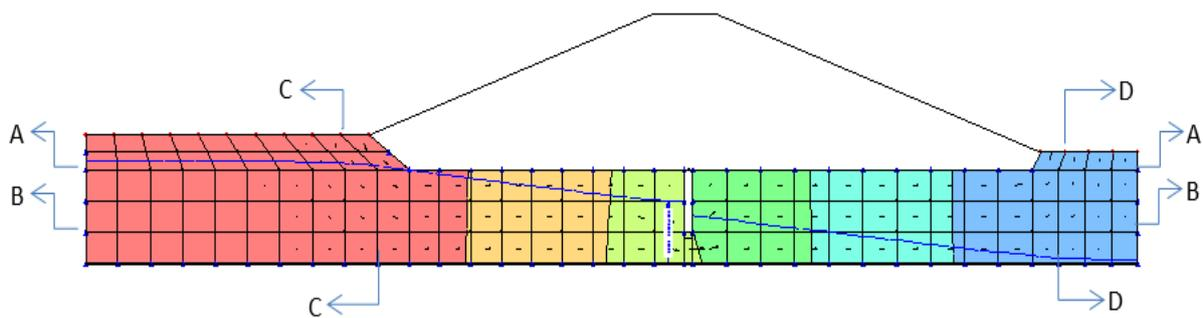
**Fig.(11):Result of Seepage Through The foundation of Al-Fada Dam**
