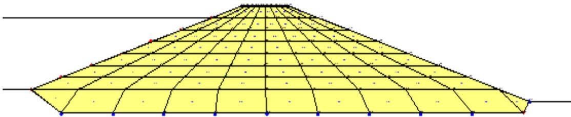
**Fig.(16): Finite Element Mesh For Al-fada Dam**
