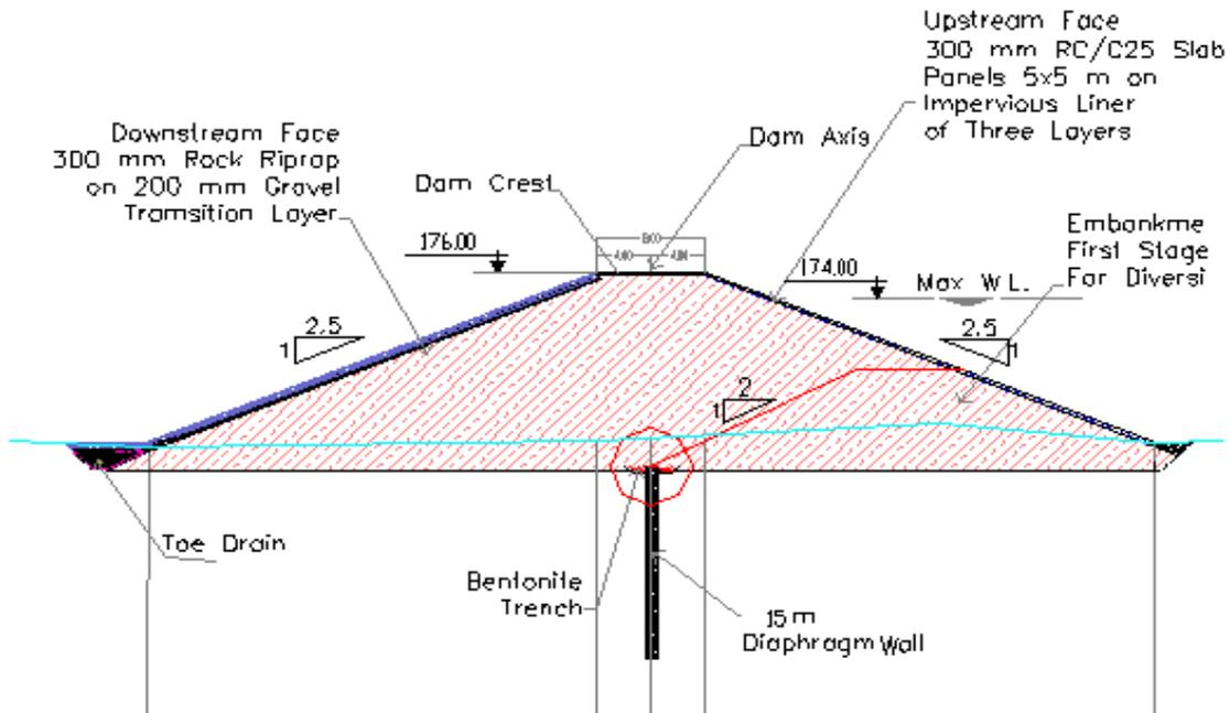
**Fig. (1) – AL-FADA Dam Typical Section**
