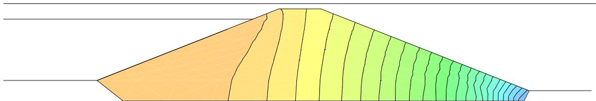
**Fig.(17):Result of Seepage Through The Body of Al-Fada Dam**
