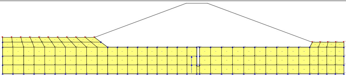
**Fig.(10):Finite Element Mesh For foundation of Al-Fada Dam**
