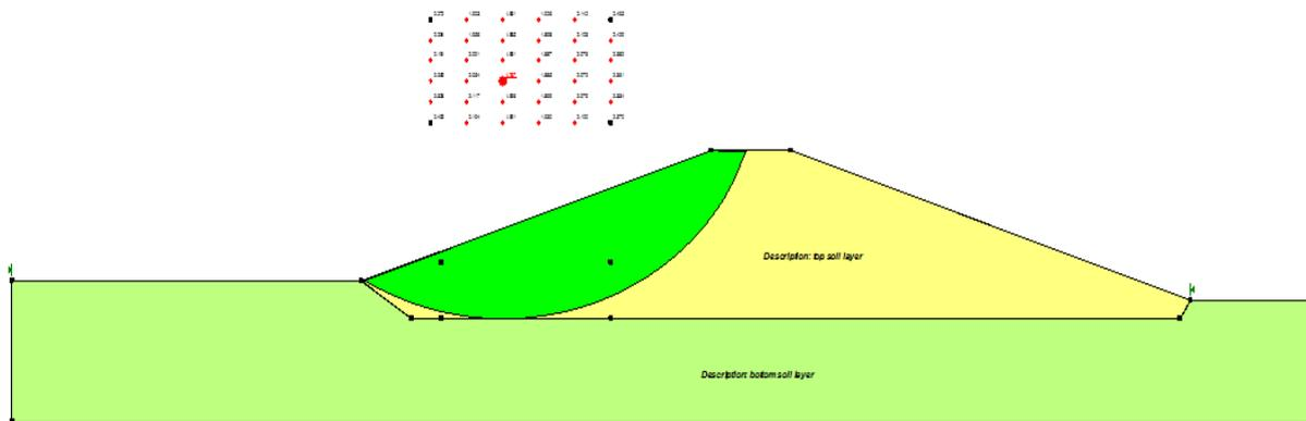
**Fig.(6):** Al-Fada Dam Case 3 -Safety Factor(1) = 1.787
