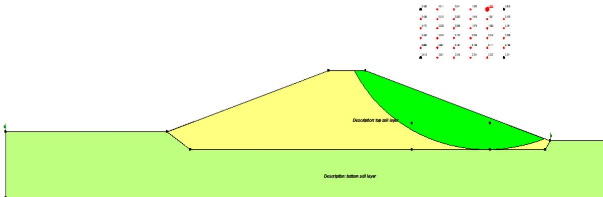
**Fig.(8): Al-Fada Dam Case 4 -Safety Factor(1) = 1.893**
