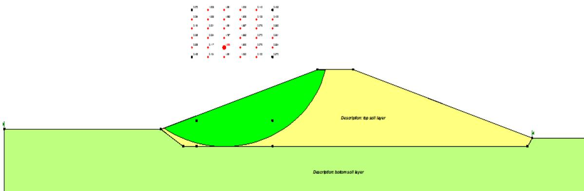
**Fig.(7):** Al-Fada Dam Case 3 -Safety Factor(2) = 1.828
