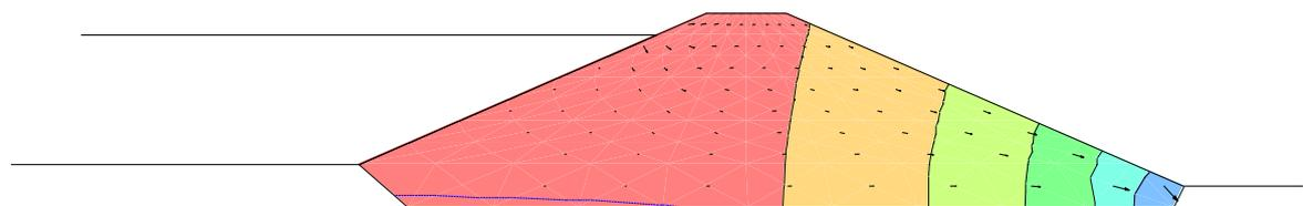
**Fig.(18):Direction of Seepage Through The Body of Al-Fada Dam**
