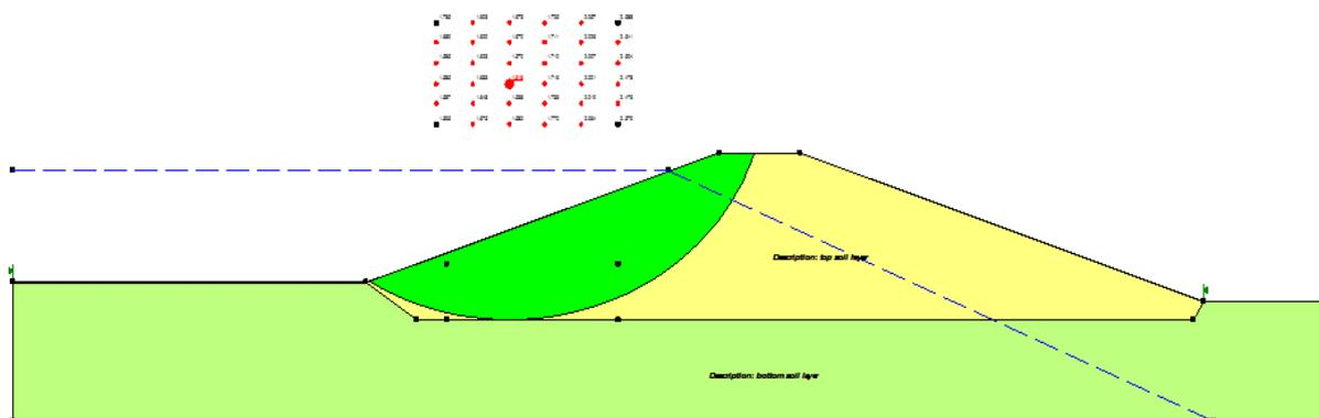
**Fig.(2): Al-Fada Dam Case 1-Safety Factor(1) = 1.516**
