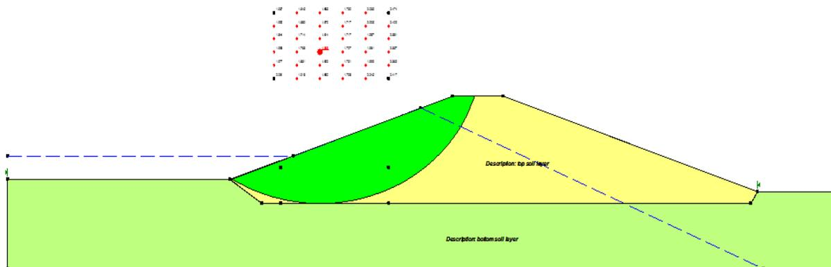
**Fig.(4): Al-Fada Dam Case 2 -Safety Factor(1) = 1.565**
