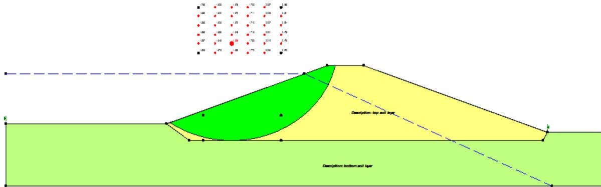
**Fig.(3): Al-Fada Dam Case 1 -Safety Factor(2) = 1.538**
