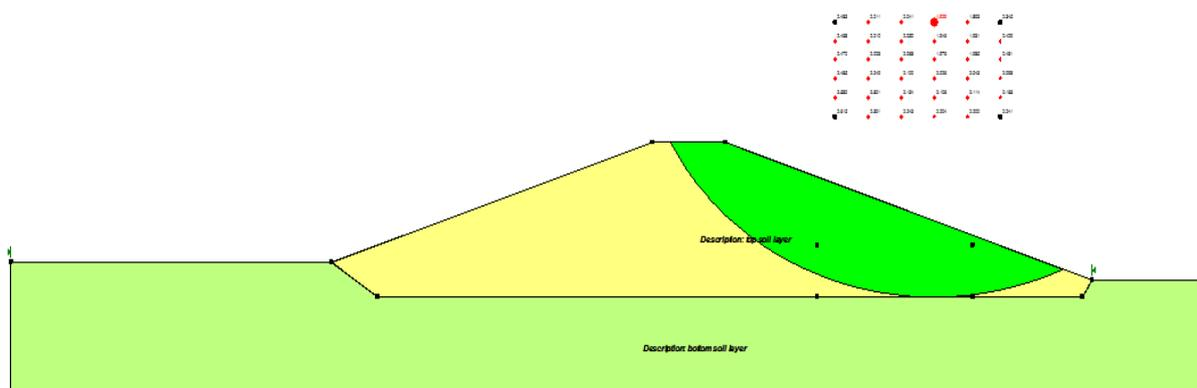
**Fig.(9): Al-Fada Dam Case 4 -Safety Factor(2) = 1.931**
