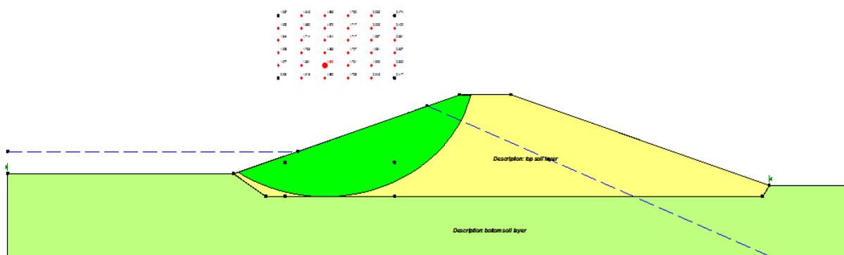
**Fig.(5): Al-Fada Dam Case 2 -Safety Factor(2) = 1.600**
