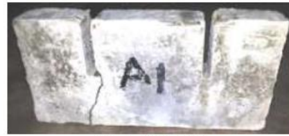
Plate (12): R1 (Group A, NWC, no waste plastic, 1 bar long. reinf. & no heat)
