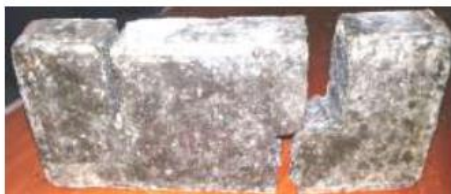
Plate (23): R0NSPH (Group D, non-structural concrete, waste plastic, 0 bars long. reinf. & subjected to heat)
