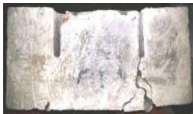
Plate (33): R2SP (Group F, structural concrete, waste plastic, 2 bars long. reinf. & subjected to heat)
