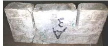
Plate (14): R3 (Group A, NWC, no waste plastic, 3 bars long. reinf. & no heat)
