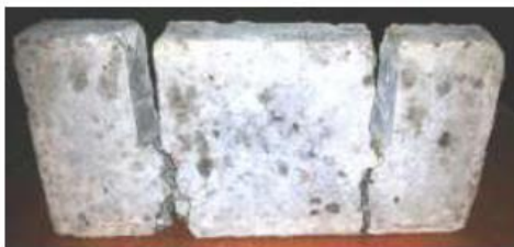
Plate (15): R0H (Group B, NWC, no waste plastic, 0 bar long. reinf. & subjected to heat)
