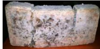
Plate (30): R3SP (Group E, structural concrete, waste plastic, 3 bars long. reinf. & no heat)
