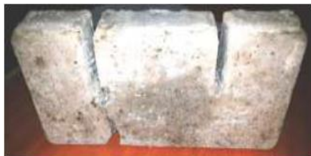
Plate (31): R0SP (Group F, structural concrete, waste plastic, 0 bars long. reinf. & subjected to heat)
