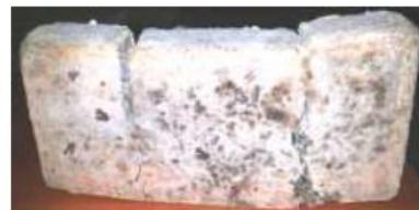
Plate (26): R3NSPH (Group D, non-structural concrete, waste plastic, 3 bars long. reinf. & subjected to heat)
