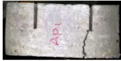
Plate (28): R1SP (Group E, structural concrete, waste plastic, 1 bar long. reinf. & no heat)
