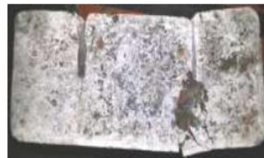
Plate (34): R3SP (Group F, structural concrete, waste plastic, 3 bars long. reinf. & subjected to heat)
