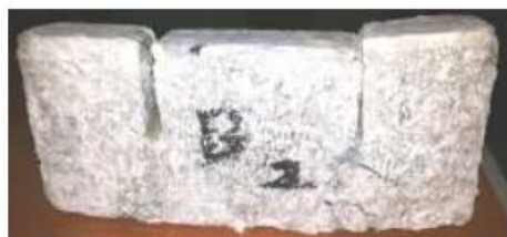
Plate (17): R2H (Group B, NWC, no waste plastic, 2 bars long. reinf. & subjected to heat)
