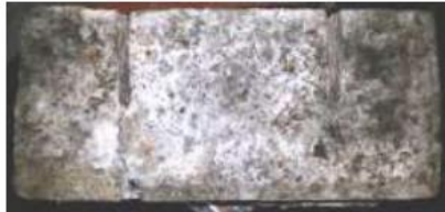
Plate (29): R2SP (Group E, structural concrete, waste plastic, 2 bars long. reinf. & no heat)
