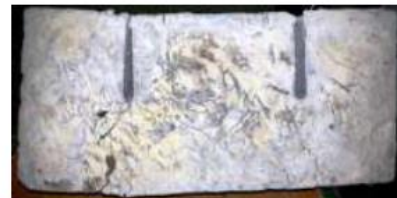
Plate (22): R3NSP (Group C, non-structural LWC, waste plastic, 3 bars long. reinf. & no heat)
