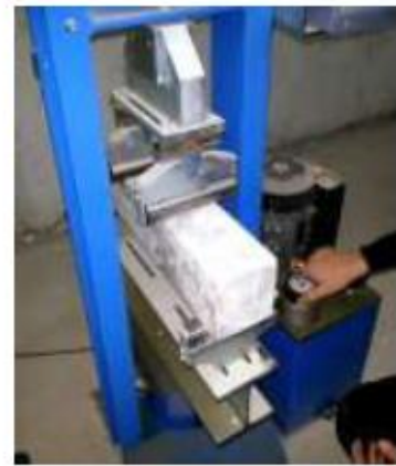
Plate(6): Flexural strength test
