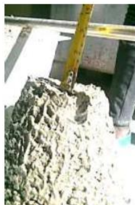
Plate (2): Slump tests
