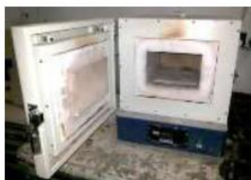
Plate (9): The electric furnace used
