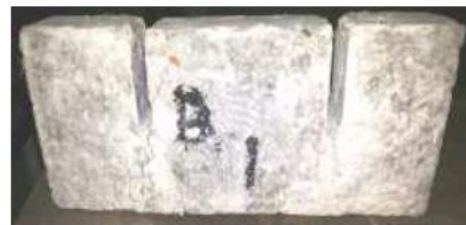
Plate (16): R1H (Group B, NWC, no waste plastic, 1 bar long. reinf. & subjected to heat)
