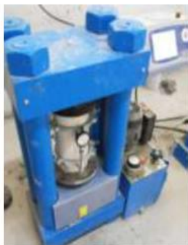
Plate (7): Concrete Modulus of Elasticity Test
