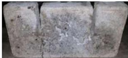
Plate (21): R2NSP (Group C, non-structural LWC, waste plastic, 2 bars long. reinf. & no heat)
