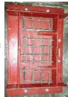
Plate (8): Typical steel mold with skin reinforcement
