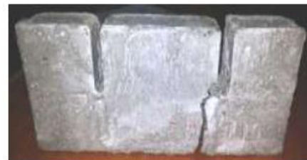
Plate (32): R1SP (Group F, structural concrete, waste plastic, 1 bar long. reinf. & subjected to heat)
