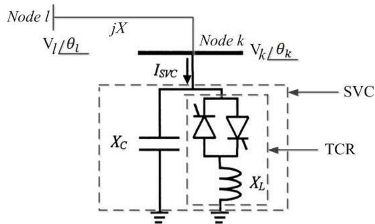
Figure 3. Equivalent circuit of SVC connected with bus k of distribution system
