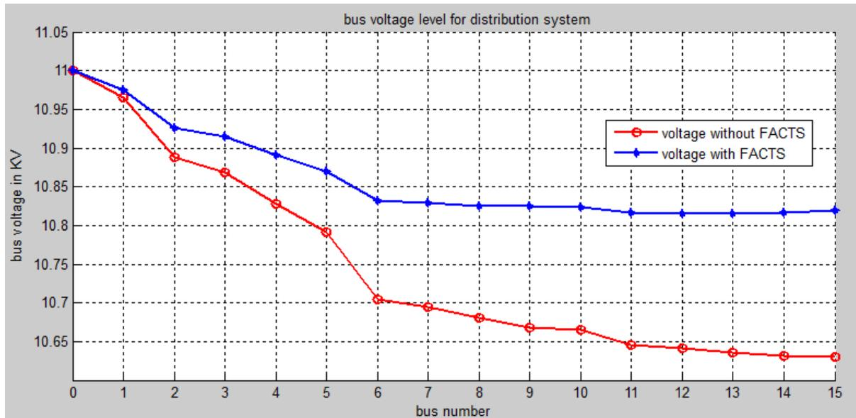
Figure 6. Voltage profile for radial distribution system (case of study)
