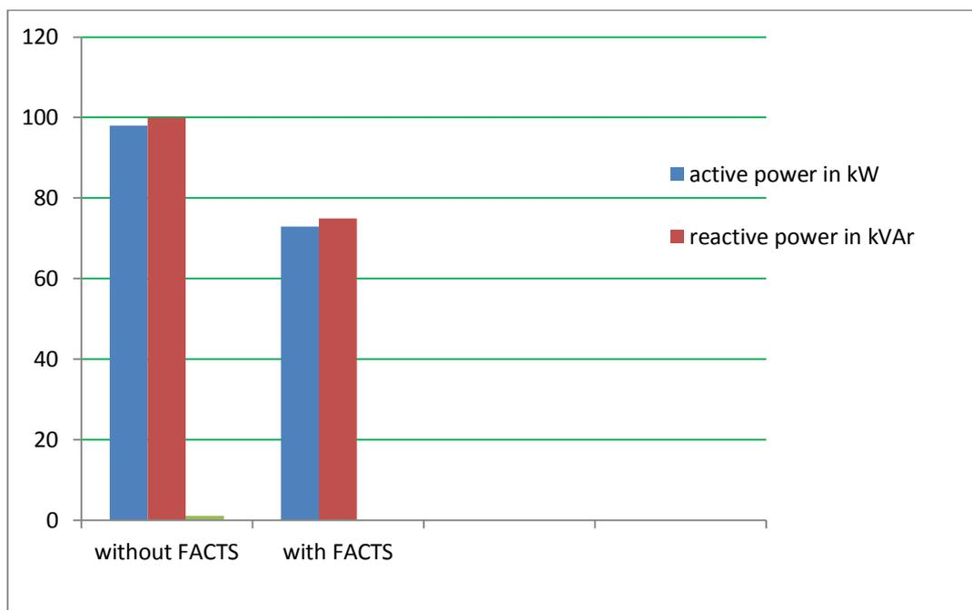
Figure 7. Total active and reactive power losses in radial distribution system (case of study)
