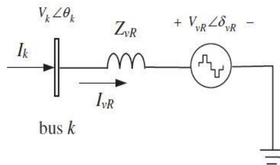
Figure 4. Equivalent circuit of static compensator (STATCOM) connected with bus k of network
