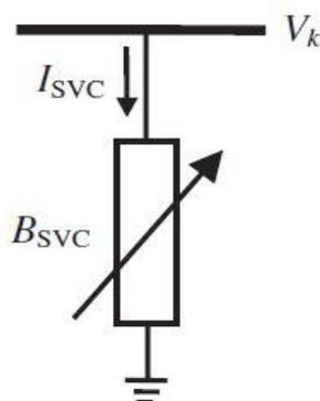
Figure 2. Variable shunt susceptance of SVC
