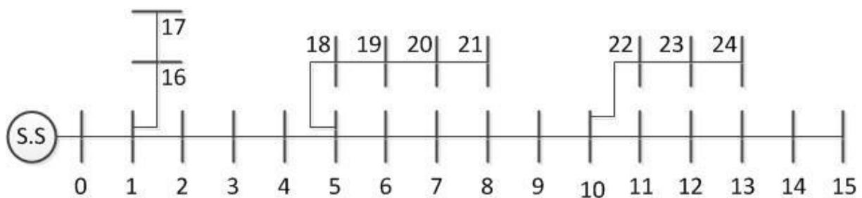
Figure 5. One line diagram for radial distribution system (case of study)
