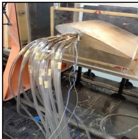
Figure 1.NACA0015 model mounted inside wind tunnel
