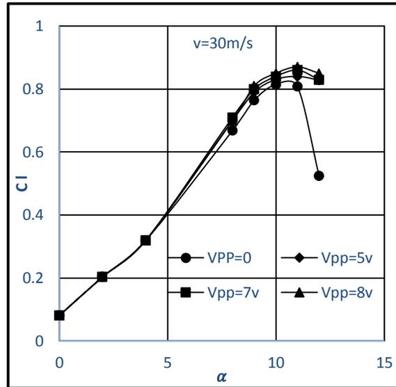
Figure 6. The comparison of computed aerodynamic coefficients experimental data at  $v_{pp}=0v$ ,  $5v$ ,  $7v$ ,  $8v$  and  $f=3.26$  kHz at  $3\%c$ .
