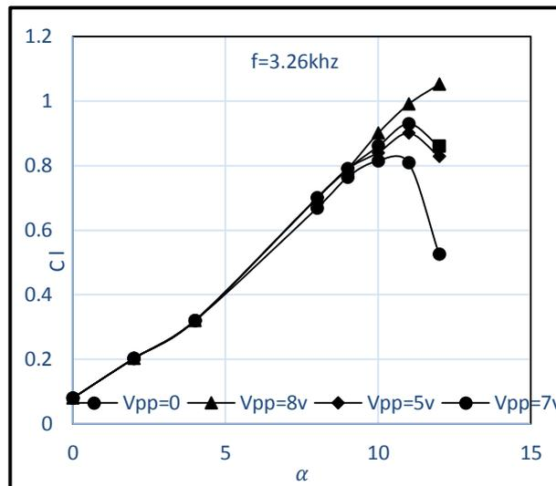
Figure 9. Comparison of lift coefficient at  $f=3.26\text{ kHz}$  and  $V_{pp} = 0, 5, 7$  and  $8$  volts at 6% c.
