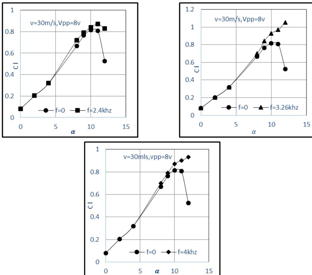
Figure 5. The lift coefficients experimental data with SJA frequency ( $f=0, 2.4, 3.26$  and  $4$  kHz) are placed at  $3\% c$ .
