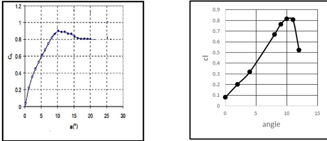
Figure 4. Comparison of experimental data for the lift coefficient over uncontrolled NACA0015 airfoil with the previous experimental data [13, 14]
