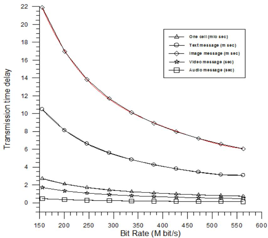
Figure (12): change in Transmission Delay Time due to changes in bit rate for one cell, text, image, video, audio message.
