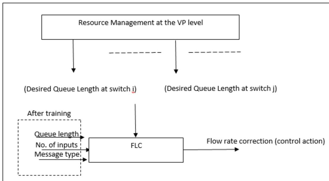
Figure (2): Block diagram of adaptive cell multiplexing controller.
