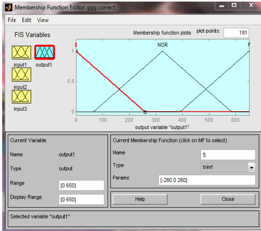
Figure (7): output variable (cell rate) membership function.
