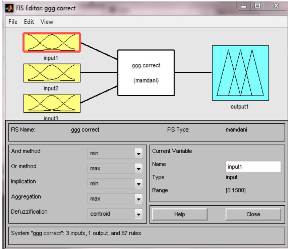
Figure (3): simulation of FLC for cell multiplexing.
