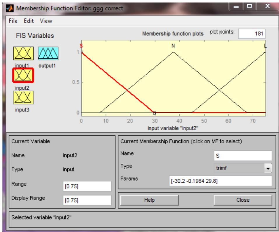
Figure (6): input variable (No. of inputs) membership function.
