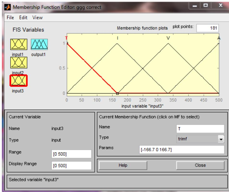
Figure (5): input variable (message type) membership function.
