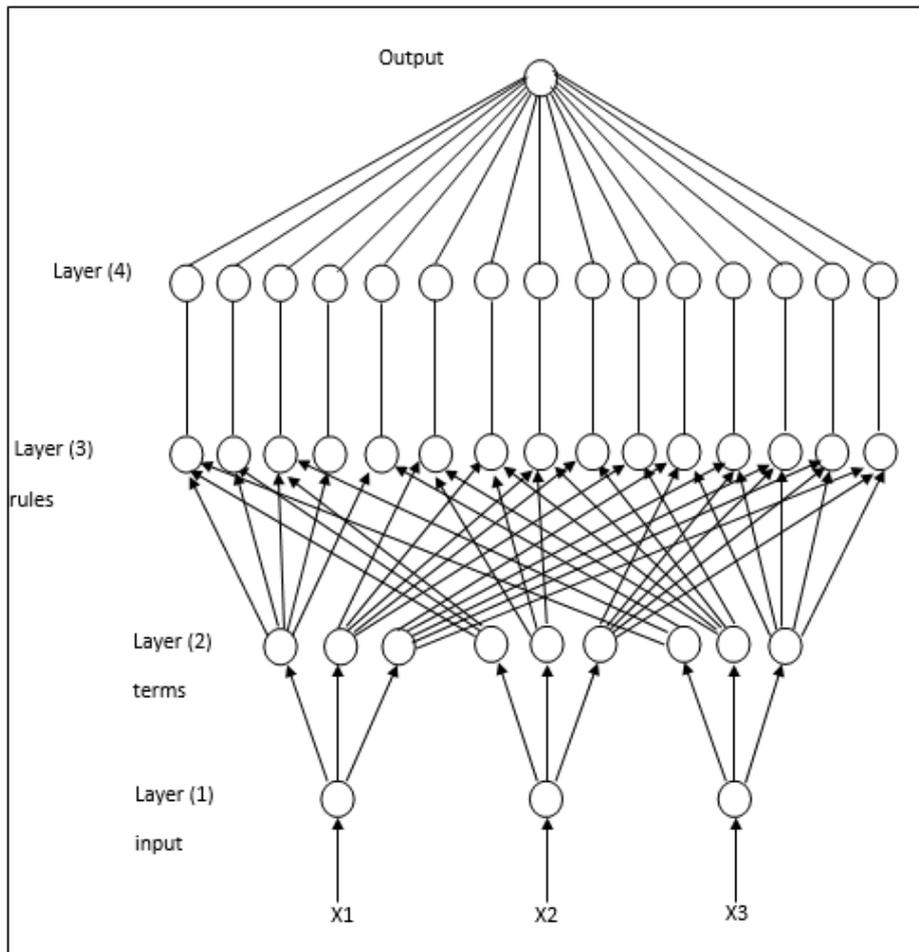
Figure (10): Adaptive neuro-fuzzy inference system architecture.
