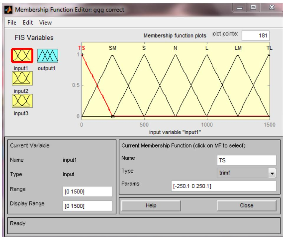
Figure (4): input variable (message length) membership function.
