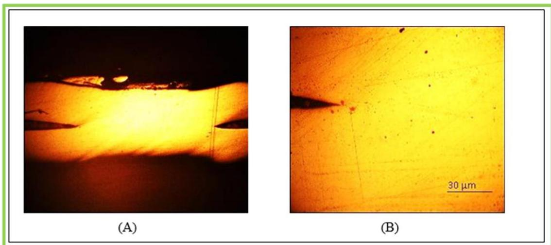
**Figure (13):** Macroetching structure for (7900 Ampere) weld specimen with different magnifications (A) 5X and (B) 10X.
