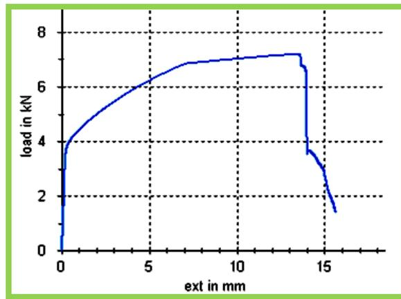
**Figure (7):** Tension test result of (7900 Amp) test specimen.
