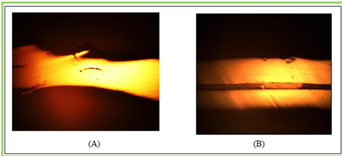
**Figure (12):** (A) 5X welding current 7300 Ampere without copper foil (B) 5X welding current 7300 Ampere with copper foil.
