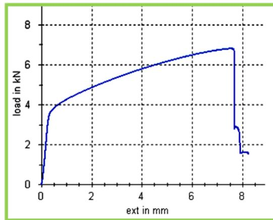
**Figure (8):** Tension test result of (7300 Amp) without copper foil.
