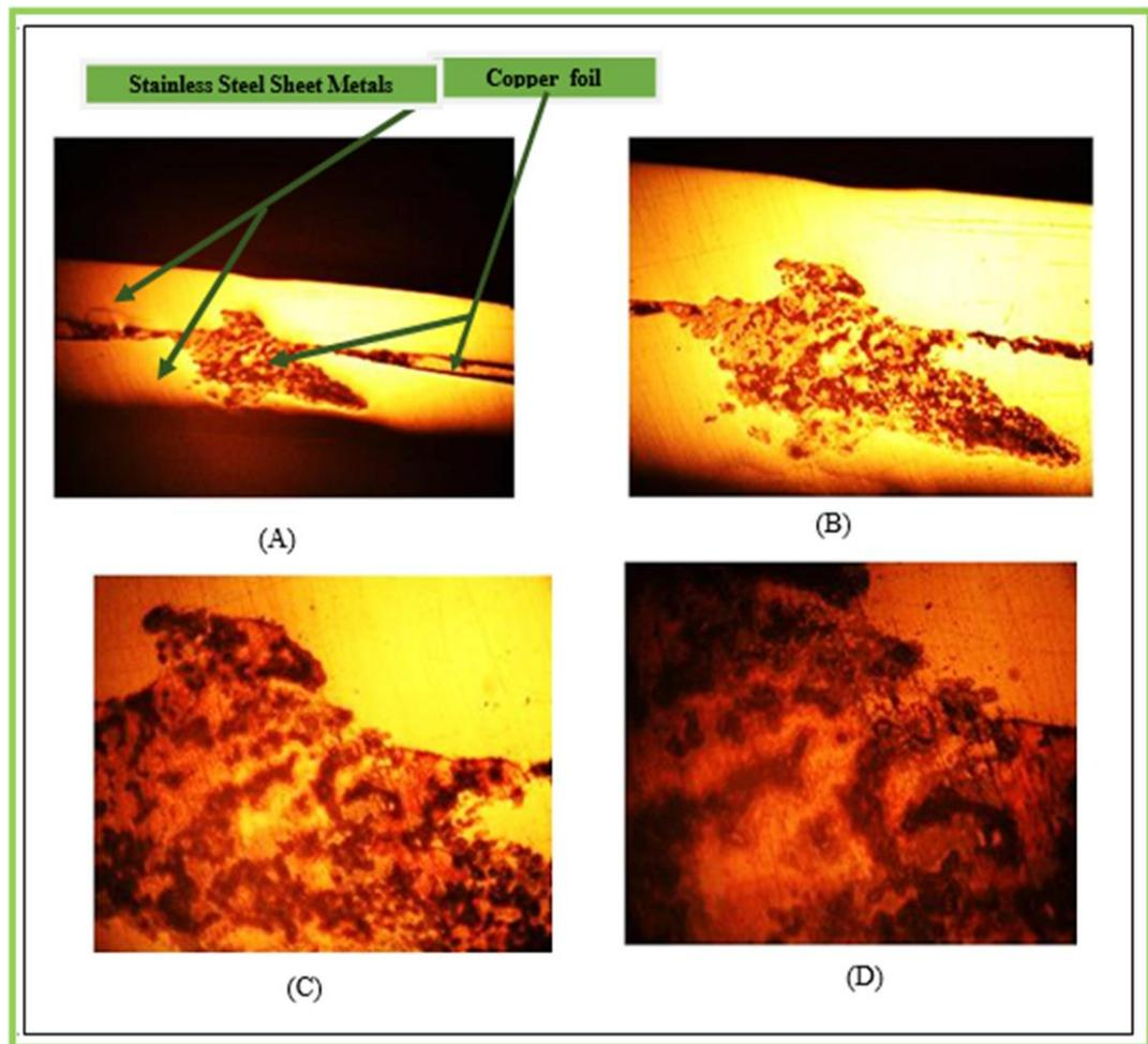
**Figure (11):** Macroetching structure for (6700 Ampere) weld specimen, with different magnifications (A) 5X, (B) 10X, (C) 20X, (D) 40X.
