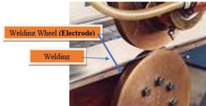
Figure (1): Resistance Seam Welding Process.
