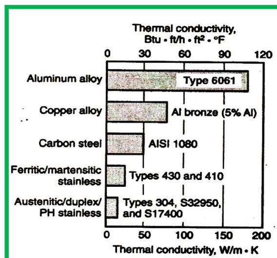
Figure (3): Comparison of thermal conductivity for copper alloy and stainless steel.
