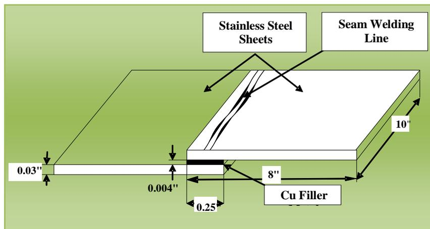
Figure (5): Standard Seam Welding Joints with Copper Filler Metal.
