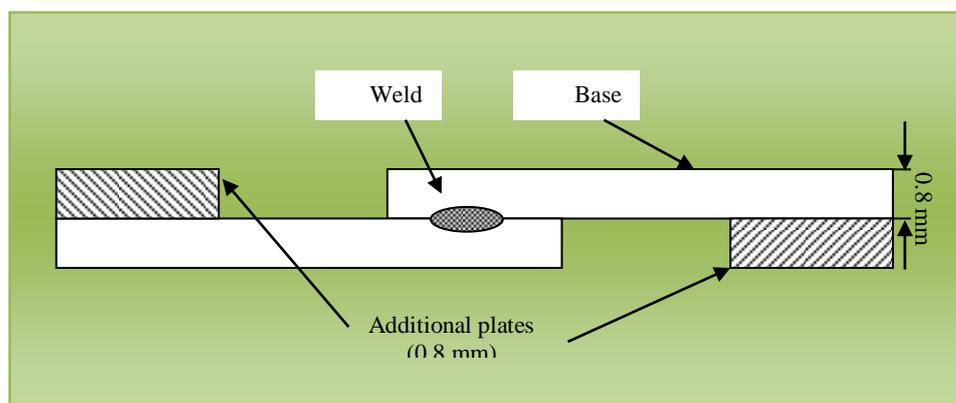
Figure (6): Standard Tension Test Specimen for Seam Welded Joints.
