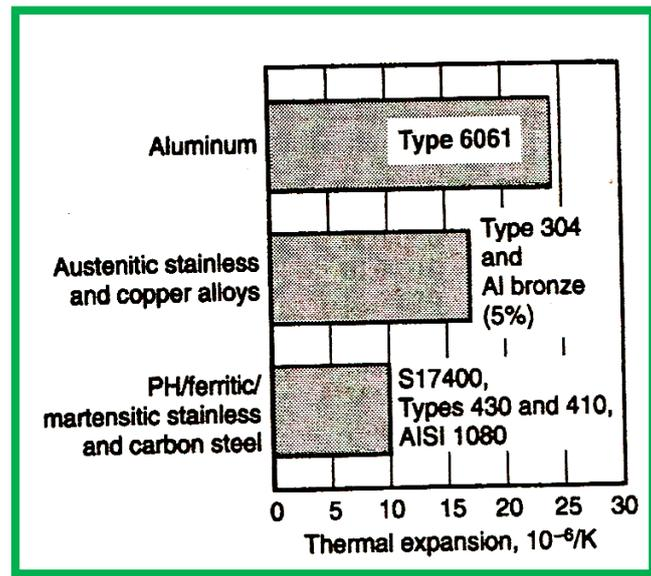
Figure (4): Comparison of thermal expansion for copper alloy and stainless steel.
