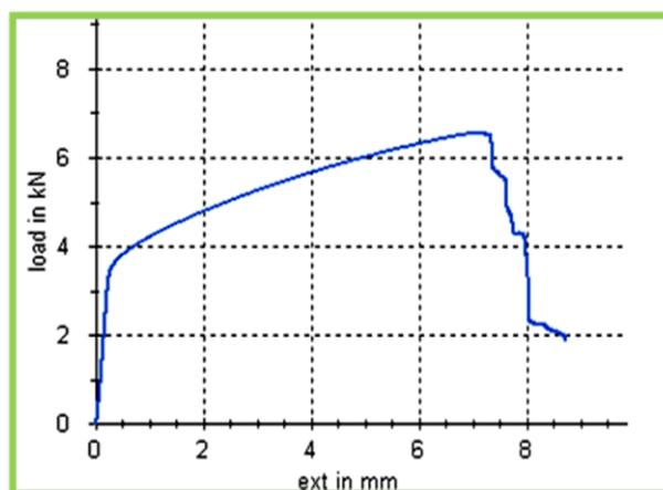
**Figure (9):** Tension test result of (6700 Amp) test specimen.
