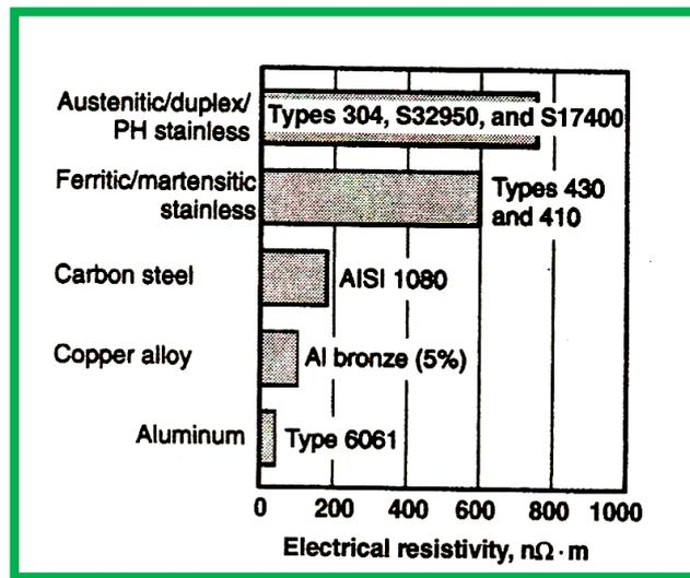
Figure (2): Comparison of electrical resistivity for copper alloy and stainless steel.
