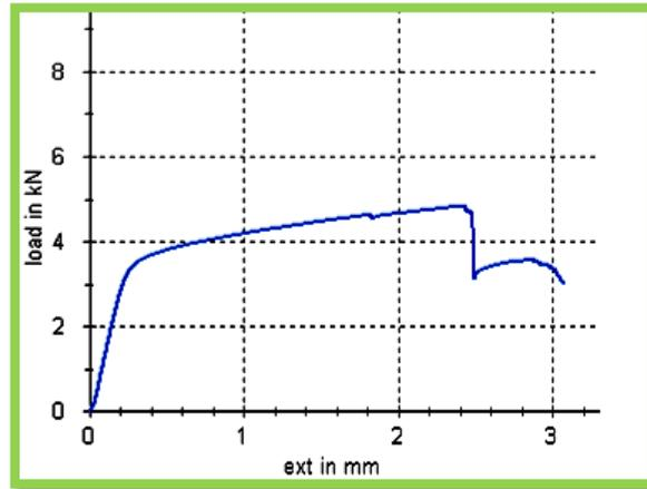
**Figure (10):** Tension test result of (9200 Amp) test specimen.
