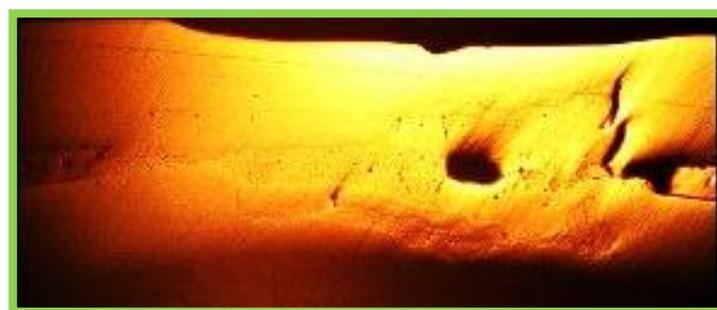
**Figure (14):** Macroetching structure for (9200 Ampere) weld specimen, with 5X magnifications.
