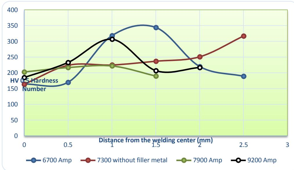
Figure (15): Micro Hardness Test Results.
