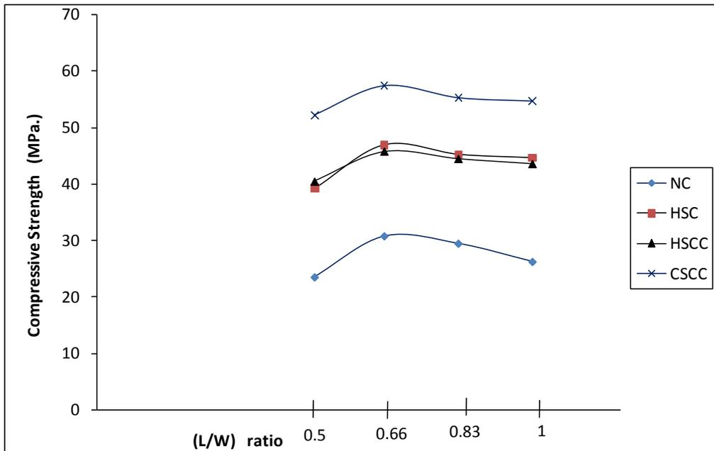
**Figure (1):** Relation between (L/W) ratio and compressive strength of (150\*150\*150) mm cubes.
