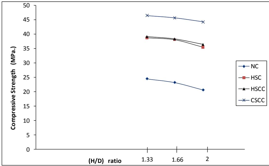
**Figure (3):** Relation between (H/D) ratio and compressive strength of (150\*300) mm cylinders.
