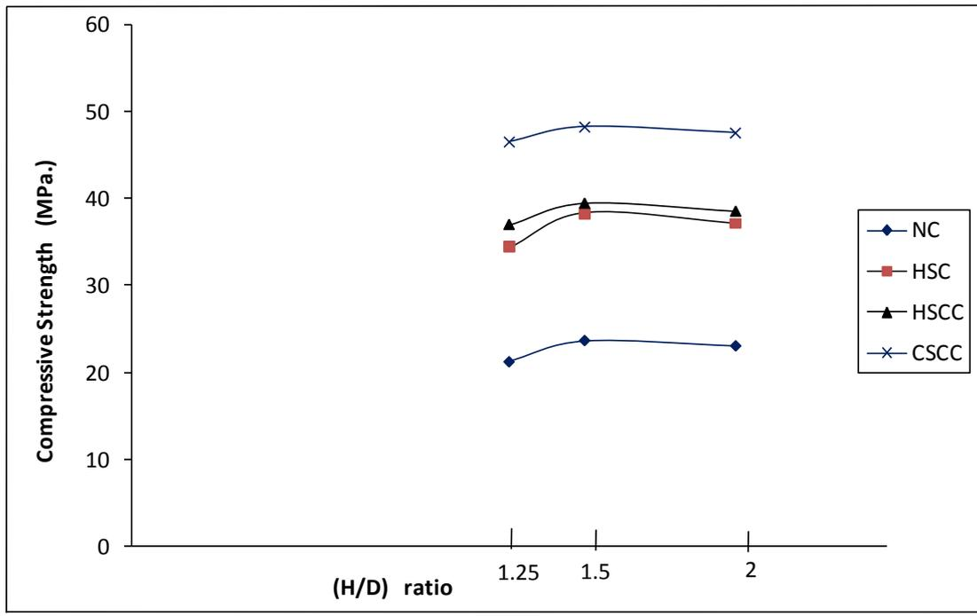
**Figure (4):** Relation between (H/D) ratio and compressive strength of (100\*200)mm cylinders.
