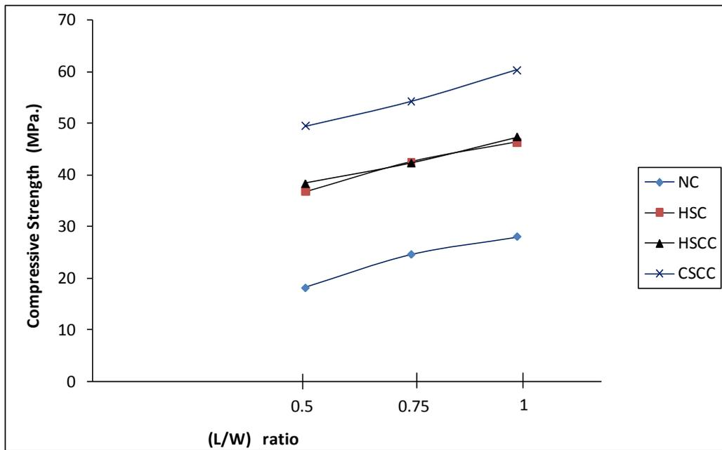
**Figure (2):** Relation between (L/W) ratio and compressive strength of (100\*100\*100) mm cubes.
