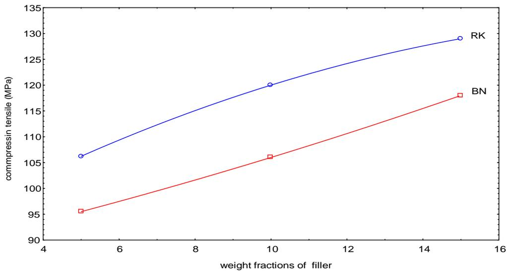
Fig. (6): The relation between compression strength of PP/PA6 with weight fraction of both RK and BN filler at temperature (25) °C
