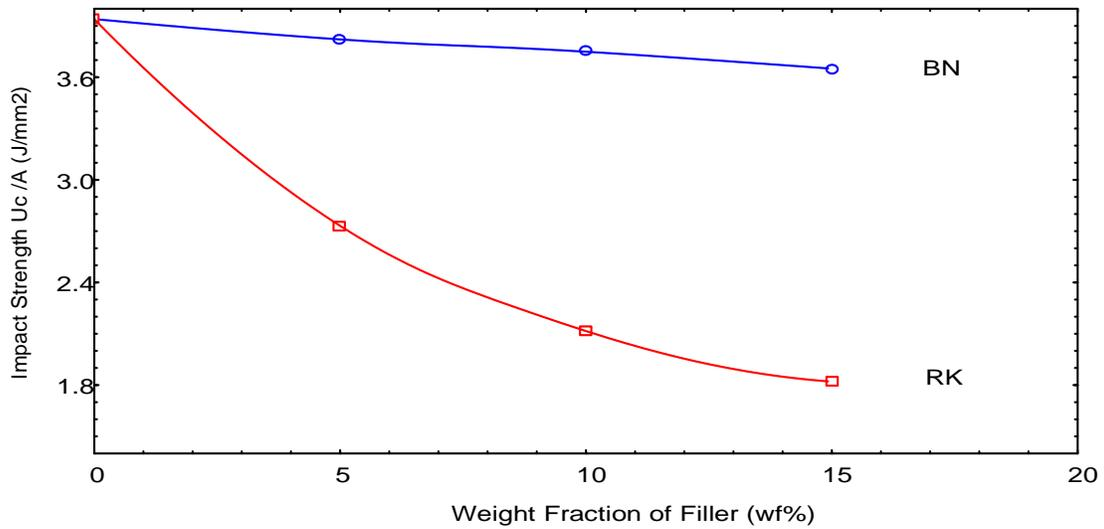
**Fig. (9):** The relation between impact strength of PP/PA6 with weight fraction of both RK and BN filler at temperature (25) °C.
