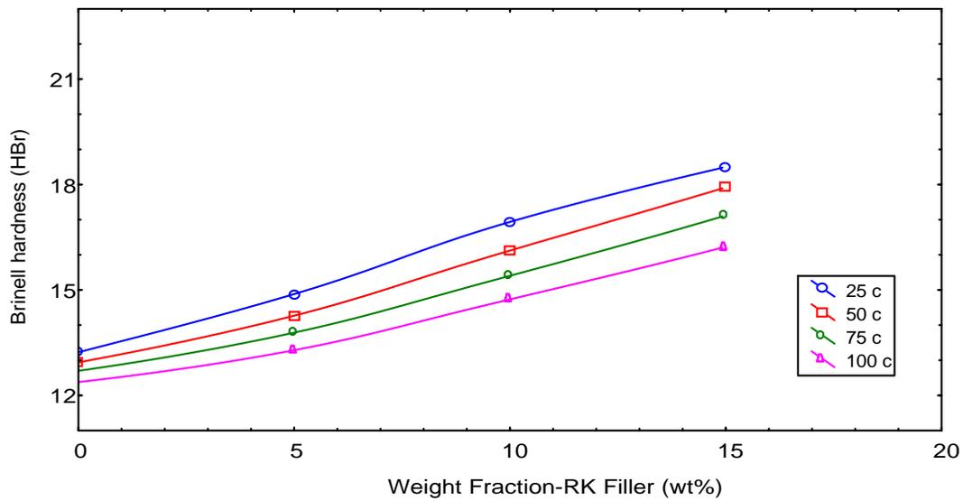
**Fig. (2):** The relation between Brinell Hardness and Weight fraction of PP/PA6/RK at different temperature (25, 50, 75,100) °C.
