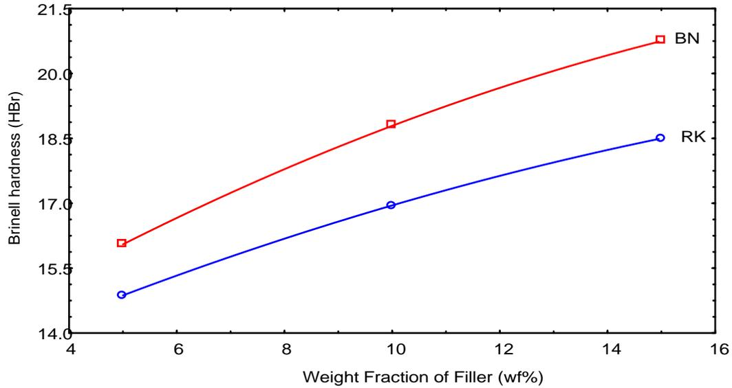
**Fig. (3):** The relation between Brinell Hardness of PP/PA6 with weight fraction of both RK and BN filler at temperature (25) °C
