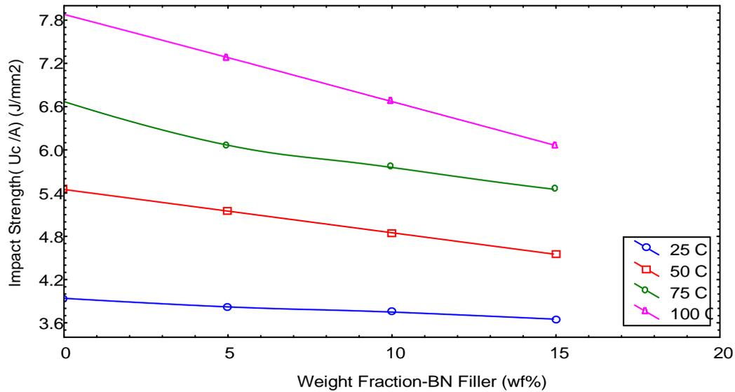
**Fig. (7):** The relation between impact strength and Weight fraction of PP/PA6/ BN at different temperature (25, 50, 75,100) °C.
