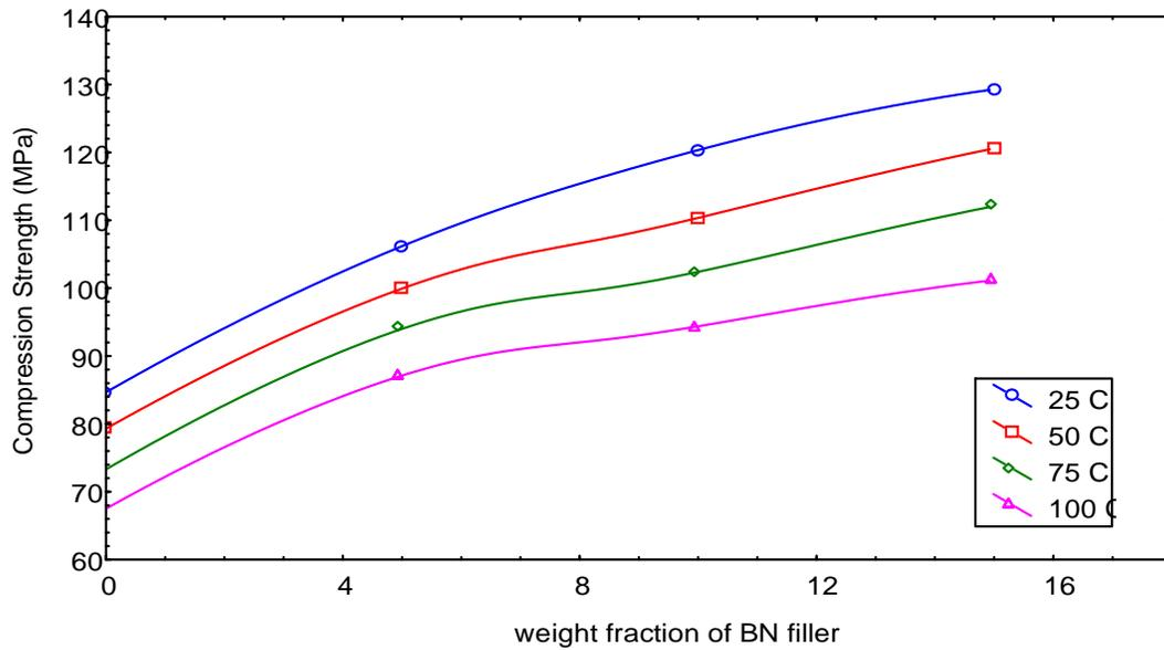
**Fig. (4):** The relation between compression strength and Weight fraction of PP/PA6/ BN at different temperature (25, 50, 75, 100) °C.
