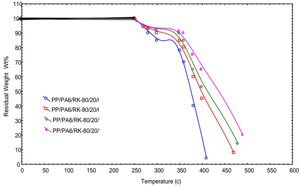
Fig. (17): Effect of addition of BN filler on thermal stability of PP/PA6 blend.
