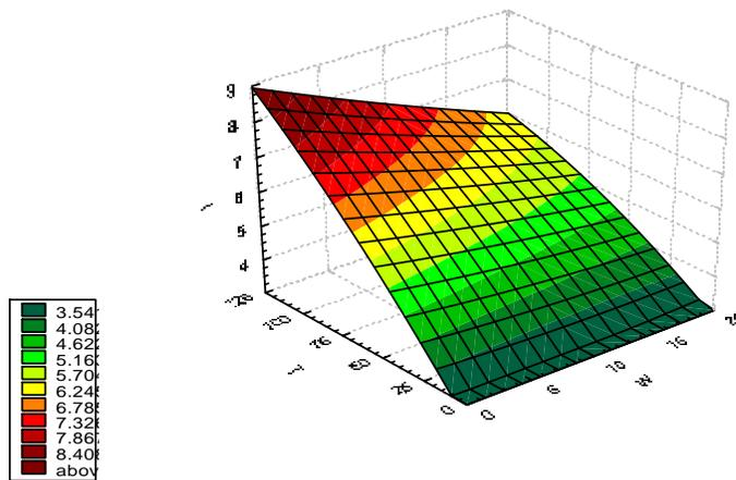
Fig. (14): Three-dimensional representation of Eq. (2) describing the variation of impact, with weight percent of filler content RK and the temperature for PP/ PA6/ RK.
