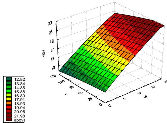
**Fig. (11):** Three-dimensional representation of Eq. (1) describing the variation of Brinell Hardness, with weight % of filler content BN and temp. for PP/PA6/BN.
