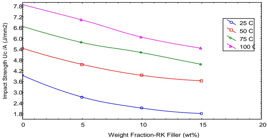
**Fig. (8):** The relation between impact strength and Weight fraction of PP/PA6/ RK at different temperature (25, 50, 75, 100) °C.
