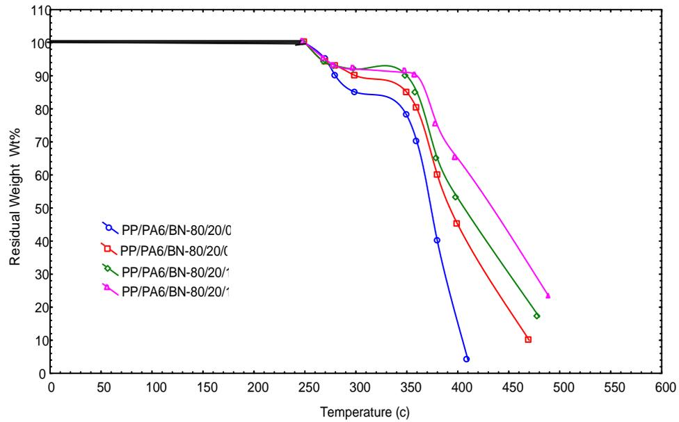
Fig. (16): Effect of addition of RK filler on thermal stability of PP/PA6 blend.
