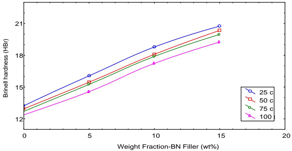
**Fig. (1):** The relation between Brinell Hardness and Weight fraction of PP/PA6/ BN at different temperature (25, 50, 75,100) °C.
