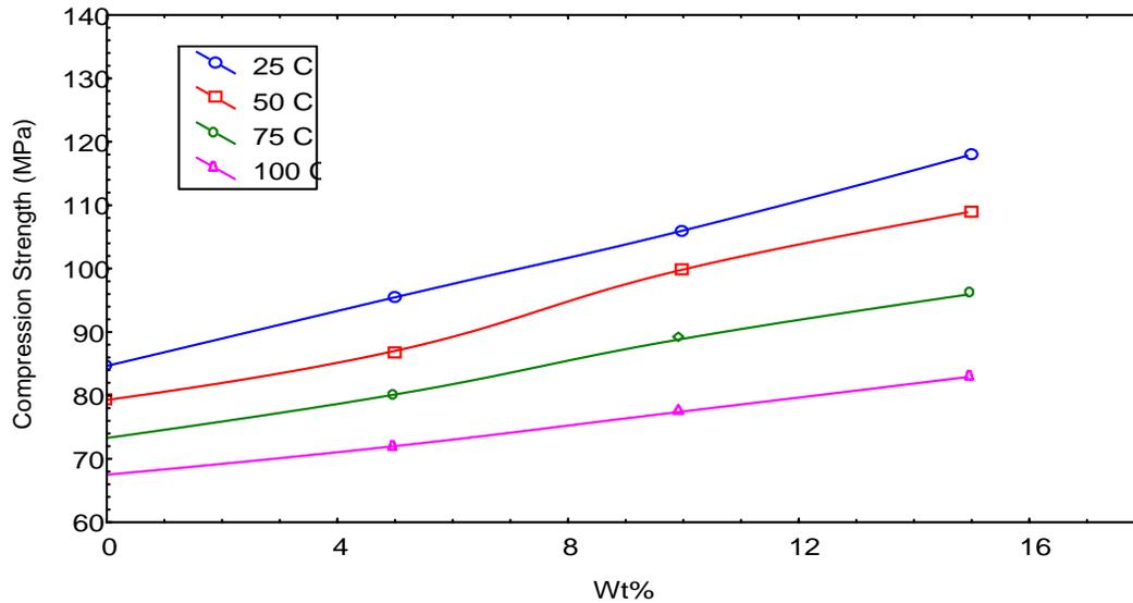
Fig. (5): The relation between compression strength and Weight fraction of PP/PA6/ RK at different temperature (25, 50, 75,100) °C.
