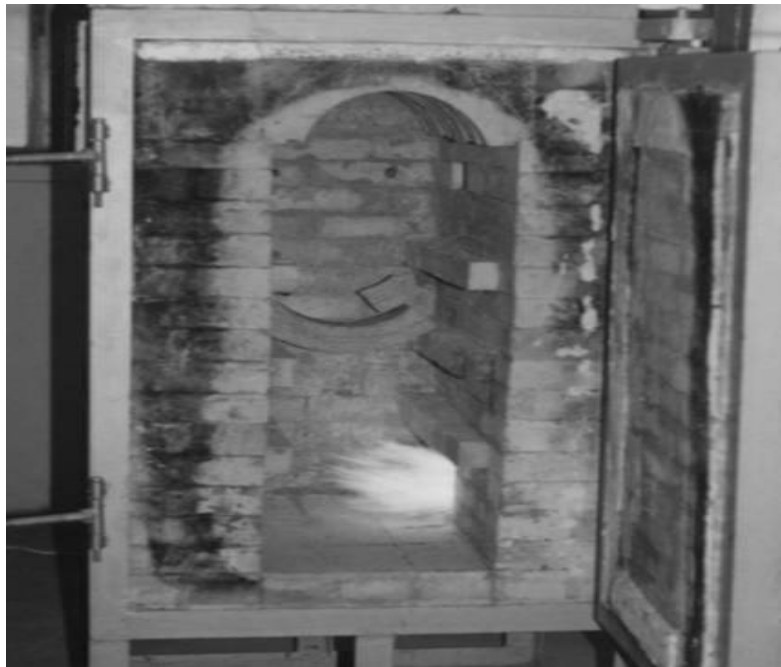
Fig.(1): Furnace at Work Showing the fire front, burning chamber, door, brick in contact with thermocouples for wall temperature measurement.
