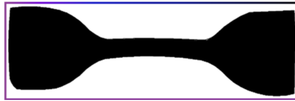
Fig. (2-a): Fatigue specimen before failure (ASTM 4484) .
